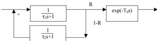
Fig. 3. Process model for MPC and Dahlin controllers.
