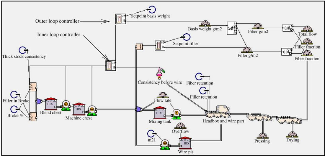
Fig. 2. Simulation model for cascade control structure.
