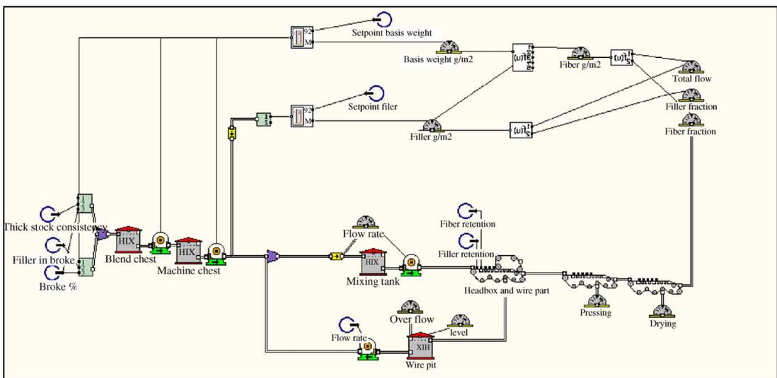
Fig. 1. Simulation model with two PI controllers. The control loops are one for filler content and one for basis weight.
