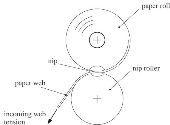
Figure 1: Winding configuration with a paper roll on top of a nip roller.
