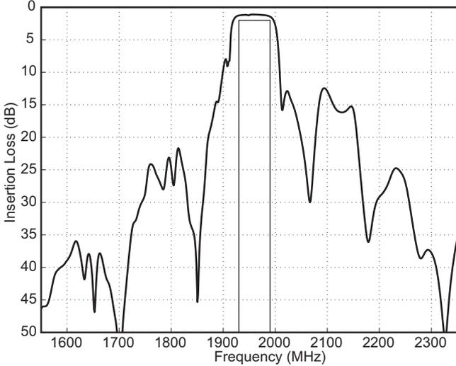
Fig. 7: Simulation of a three-transducer design with distributed gaps on  $42^\circ\text{-LiTaO}_3$ . The passband is slightly wider than in the metallized-gap design due to minimized gap loss.
