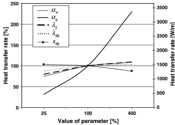
Fig. 6. The effect of some parameters on the heat transfer rate of an element (plate + fin). The assumed typical values at point 100% are  $\alpha_g = 25 \text{ W m}^{-2} \text{ K}^{-1}$ ,  $\alpha_w = 500 \text{ W m}^{-2} \text{ K}^{-1}$ ,  $\lambda_f = 52 \text{ W m}^{-1} \text{ K}^{-1}$ ,  $\lambda_{dg} = 0.1 \text{ W m}^{-1} \text{ K}^{-1}$ ,  $s_{dg} = 0.25 \text{ mm}$ ,  $s_{dw} = 0 \text{ mm}$ .
