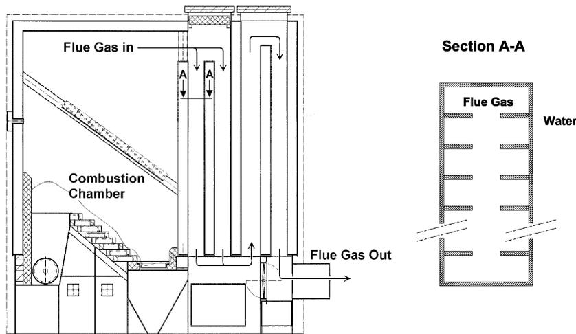
Fig. 1. The boiler Arimax BIO of Thermia Ltd. and a section of a flue gas duct in the convection section.
