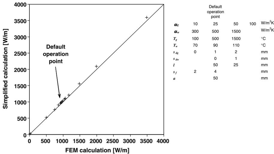
Fig. 4. A comparison between the heat transfer rates according to the FEM calculation and the assumption  $\lambda_{f,y} = \infty$  (simplified calculation, plate at uniform temperature) when changing initial parameters.
