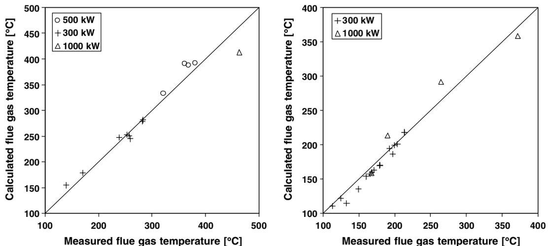
Fig. 8. A comparison between measured and calculated final flue gas temperatures of the first pass (on the left) and other passes (on the right) of the convection section. In the calculations  $s_{dg} = s_{dw} = 0$  mm.
