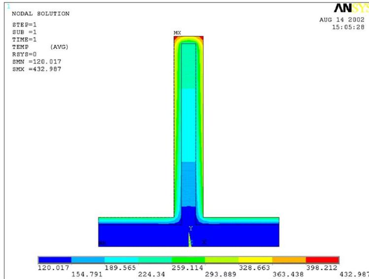
Fig. 5. A comparison of the heat transfer rate of a fouled fin between FEM and the assumption  $\lambda_{f,y} = \infty$  (above) and the corresponding temperature field using the FEM calculation (below). The data for fouling is  $s_{dg} = 2$  mm,  $s_{dw} = 0$  mm,  $\lambda_{dg} = 0.12$  W K<sup>-1</sup> m<sup>-1</sup>, other initial data is similar to the data in Fig. 3.
