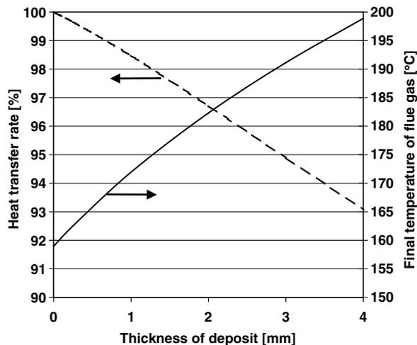
Fig. 7. The relative heat transfer rate of the convection section and the final temperature of flue gas as a function of thickness of the deposit.
