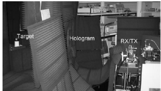
Figure 3. Test RCS measurement facility.
