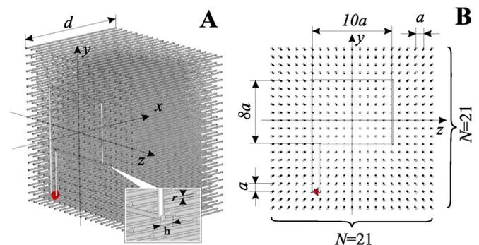
FIG. 1. (Color online) Geometry of the flat lens formed by the wire medium and the source of the form of the letter P. (A) Perspective view. (B) Front view. Parameters:  $a=10$  mm,  $r=1$  mm,  $d=150$  mm,  $h=5$  mm,  $f=1$  GHz.
