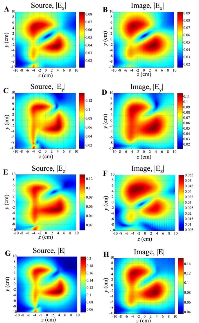
FIG. 4. (Color online) Results of near field scan measurements: absolute values of *x*-, *y*-, and *z*-electric field components and total field in arbitrary units: (A,C,E,G) in the source plane and (B,D,F,H) in the image plane, respectively.
