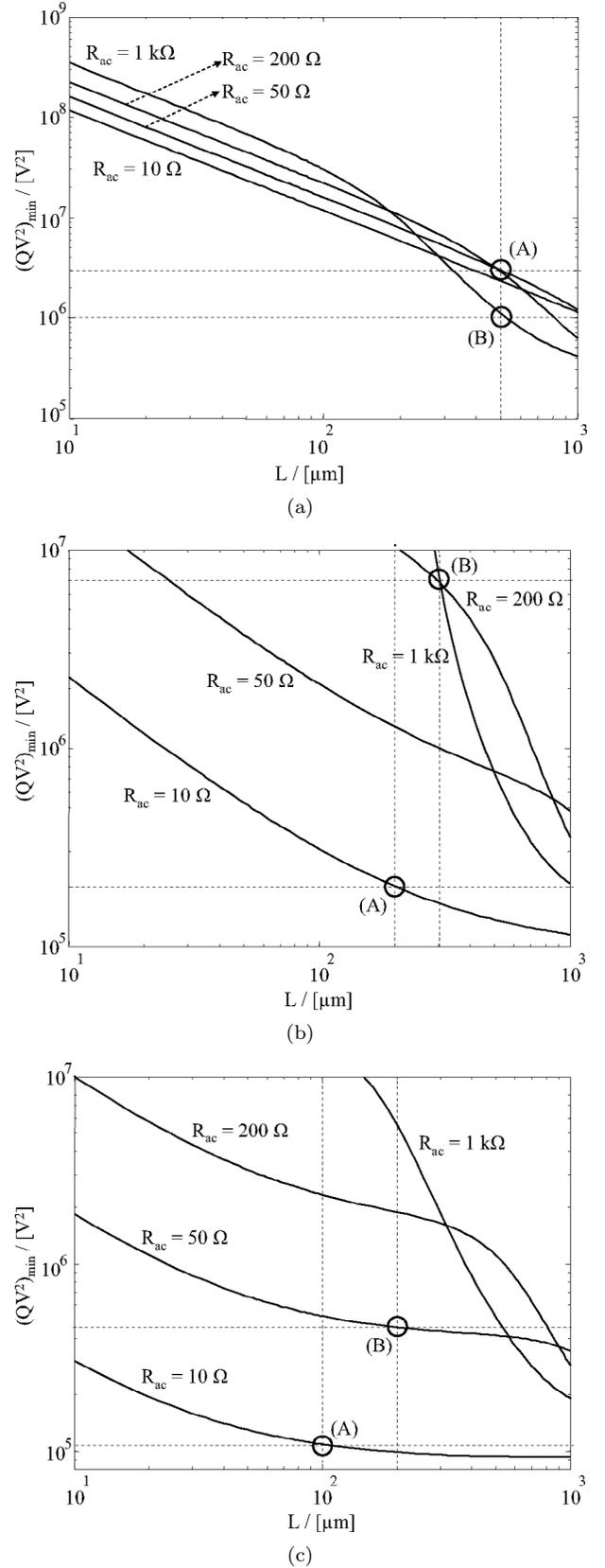
Fig. 6. Minimums of  $QV_{\text{bias}}^2$  (16), determined by the maximum in-band loss of the filter, corresponding to the resonator geometries of Fig. 5 with  $d(L) = d_{\min} + 3 \text{ nm}$ . The circles labeled (A) and (B) correspond to the designs of Table V. (a) Resistive load ( $C_L = 0$ ,  $R_L = R_{\text{ac}}$ ); (b) capacitive load ( $C_L = 1 \text{ pF}$ ,  $R_L = 1 \text{ M}\Omega$ ); (c) capacitive load ( $C_L = 0.1 \text{ pF}$ ,  $R_L = 1 \text{ M}\Omega$ ).
