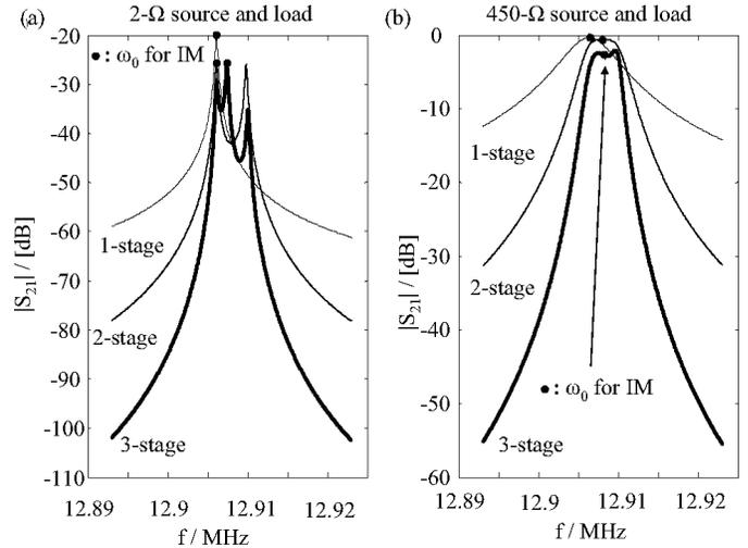
Fig. 2. Unloaded (a) and loaded (b) responses of the filters composed of one, two, and three BAW resonators, as shown in Fig. 1. The desired-user frequency  $\omega_0$  for the SIR results of Fig. 3 is marked with a dot.
