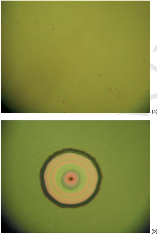
**Fig. 8** Optical micrograph of SiO<sub>2</sub> surface after post CMP cleaning: (a) overall view, (b) close up of a hole.
