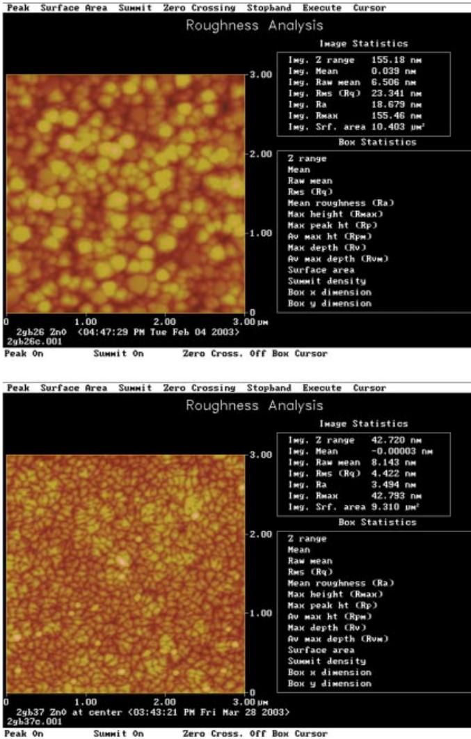
Fig. 10 AFM nanographs of ZnO surface after sputter deposition: (a) non-CMP (b) CMP smoothing applied to SiO<sub>2</sub>.
