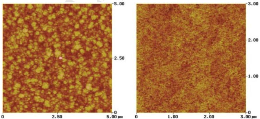
Fig. 7 AFM nanographs of SiO<sub>2</sub>: (a) before and (b) after CMP smoothing.
