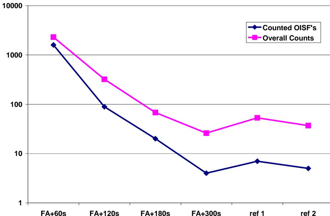
**Figure 3:** OISF counts on a diameter scan after different final polishing times. The count decreases rapidly with increasing the final polishing time and reaches reference level after 300s referring to 0.5 μm removal.
