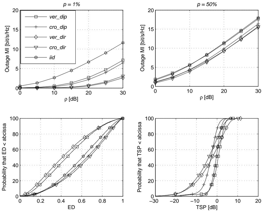
Figure 12. Four  $2 \times 2$  MIMO systems are analyzed in the indoor case. Results of outage MI, ED and TSP are considered at different subplots. Analysis of outage MI is presented in the capacity outage probability levels ( $p$ ) of 1% and 50% as a function of  $\rho$  in the upper figures. The cdfs of ED and TSP are presented in the lower figures.
