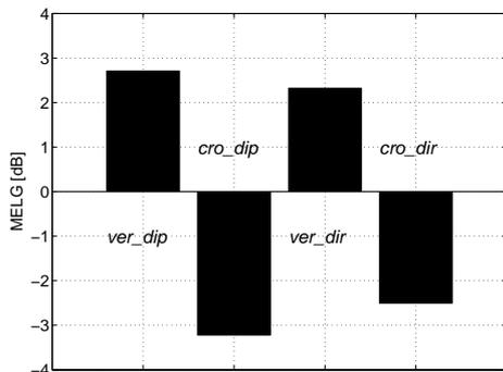
Figure 8. Results of mean effective link gain (MELG) presented for the considered antenna systems in the microcell (LOS) scenario.
