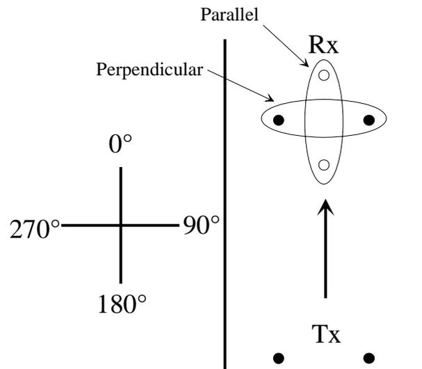
Figure 4. Rx antenna array orientations relative to Tx antenna array orientation as arranged in the microcell (LOS) environment. Patch antenna elements of the Tx antenna array are pointing to the direction of  $0^\circ$ .
