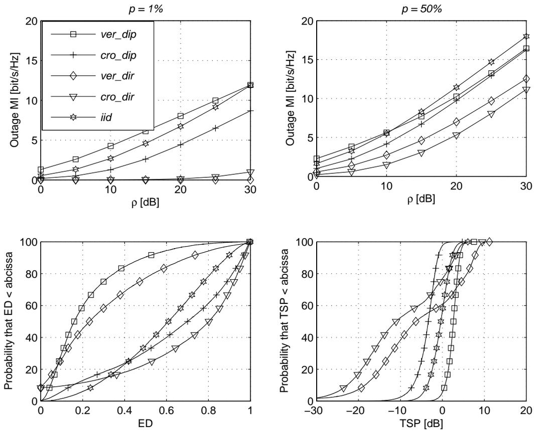
Figure 11. Four 2×2 MIMO systems are analyzed in the microcell (LOS) case. Results of outage MI, ED and TSP are considered at different subplots. Analysis of outage MI is presented in the capacity outage probability levels ( $p$ ) of 1% and 50% as a function of  $\rho$  in the upper figures. The cdfs of ED and TSP are presented in the lower figures.
