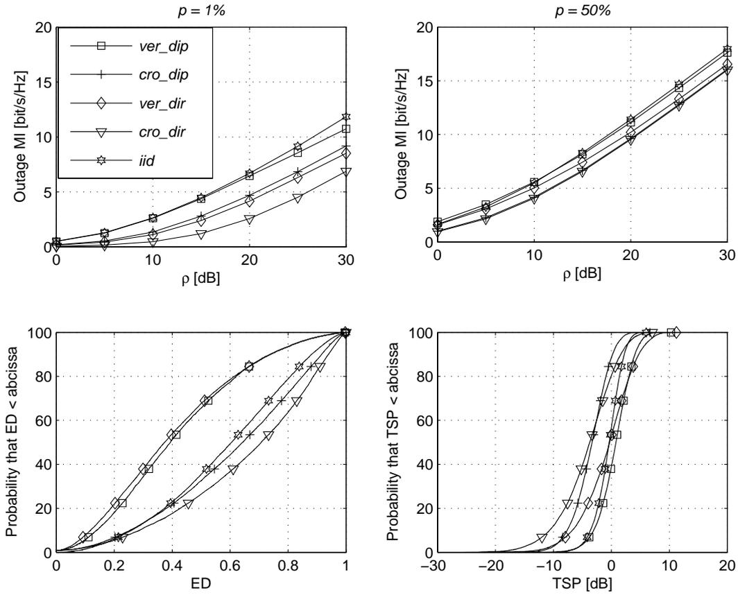
Figure 10. Four  $2 \times 2$  MIMO systems are analyzed in the small macrocell (NLOS) case. Results of outage MI, ED and TSP are considered at different subplots. Analysis of outage MI is presented in the capacity outage probability levels ( $p$ ) of 1% and 50% as a function of  $\rho$  in the upper figures. The cdfs of ED and TSP are presented in the lower figures.
