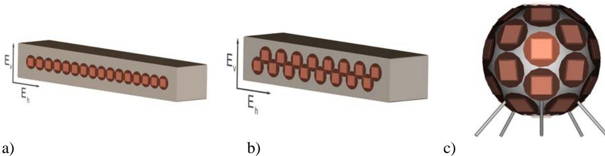
Figure 1. Antenna arrays used in measurements: a) linear (Tx), b) zigzag (Tx), c) spherical (Rx).
