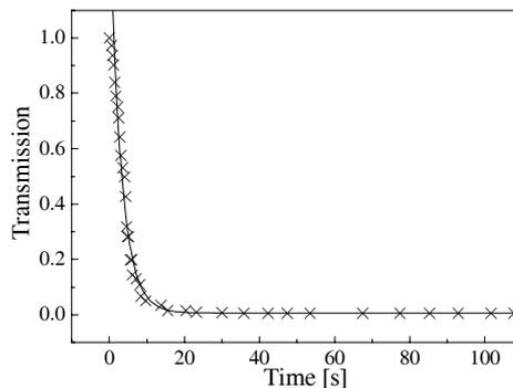
Fig. 5. Normalized transmission of  $^{12}\text{C}_2\text{H}_2$  line at 1521.060 nm as a function of time in PBF1500 recorded using a tunable laser while filling the fiber with gas to 113 mbar.
