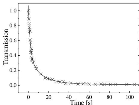
Fig. 4. Normalized transmission of  $^{12}\text{C}_2\text{H}_2$  line at 1531.588 nm as a function of time in PBF1500 recorded using a tunable laser while filling the fiber with gas to 10 mbar.
