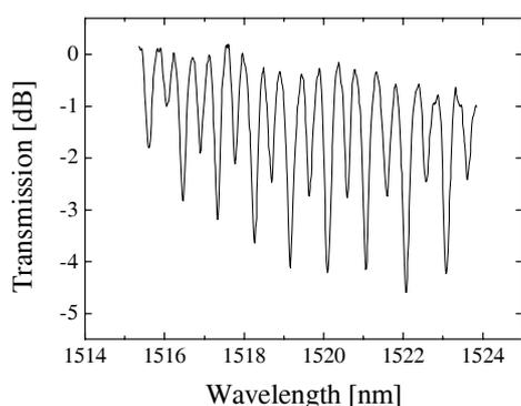
Fig. 8. Normalized absorption spectra of R-branch of  $^{12}\text{C}_2\text{H}_2$  in a 1 m long PBF1500 measured using a LED. The resolution of the OSA is 0.1 nm. The lines appear broader due to the limited resolution of the OSA.
