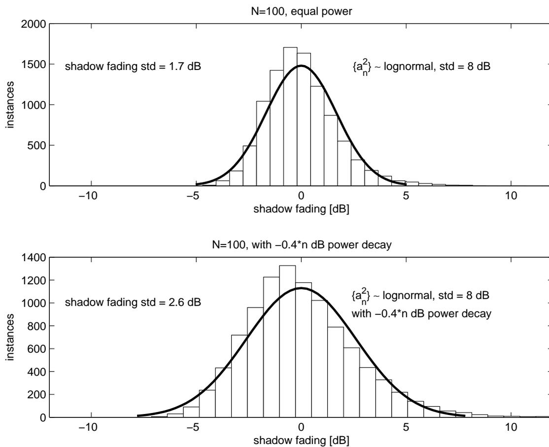
Fig. 2. Example of shadow fading distribution resulting from  $N = 100$  plane waves. The x-axis shows  $10 \log_{10}(\mathcal{P}_N)$ . The plane wave powers are distributed as  $\{b_n Y_n\}_{n=1}^N$ , where  $\{Y_n\}_{n=1}^N$  are iid lognormal random variables with zero-mean and 8 dB standard deviation. In the upper plot,  $\{b_n\}_{n=1}^N = 1$ . In the lower plot,  $10 \log_{10}(b_n) = -0.4n$  dB,  $n = 0, \dots, 99$ . The best-fit Gaussian is shown for reference.
