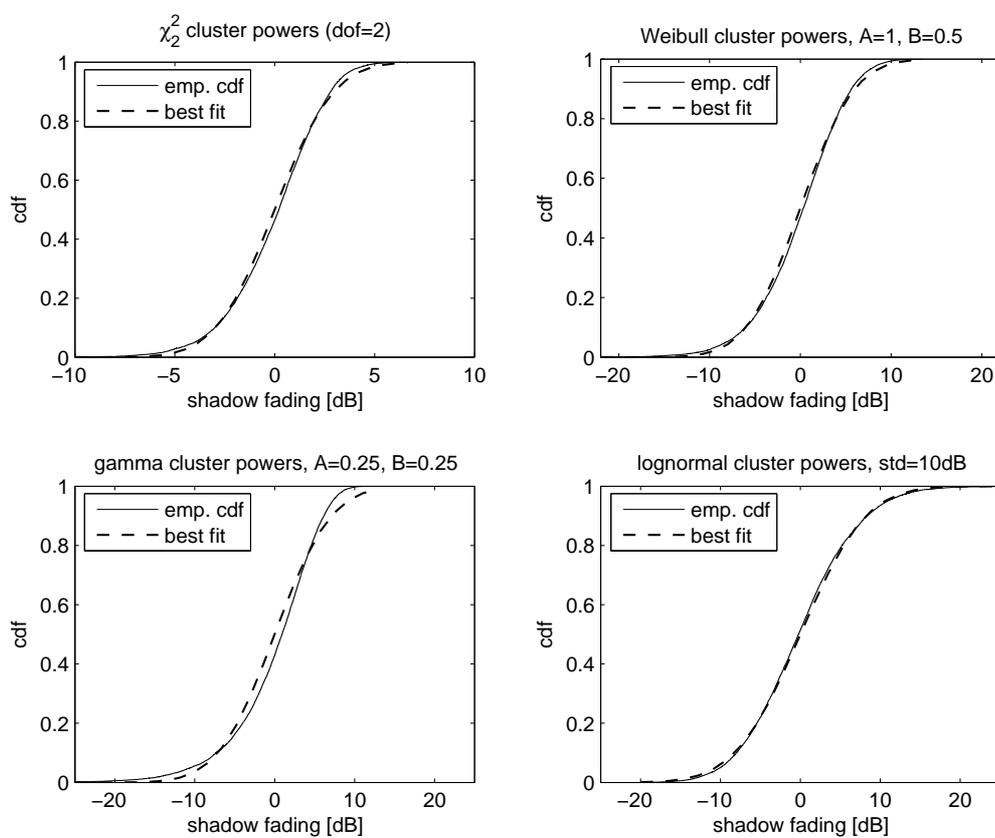
Fig. 5. Examples of shadow fading distributions resulting from different cluster power distributions. In all cases the number of clusters is four ( $K = 4$ ), and the cluster powers  $\{\mathcal{W}_k^2\}_{k=1}^K$  have iid pdfs. The best-fit Gaussian pdf is also shown for comparison.
