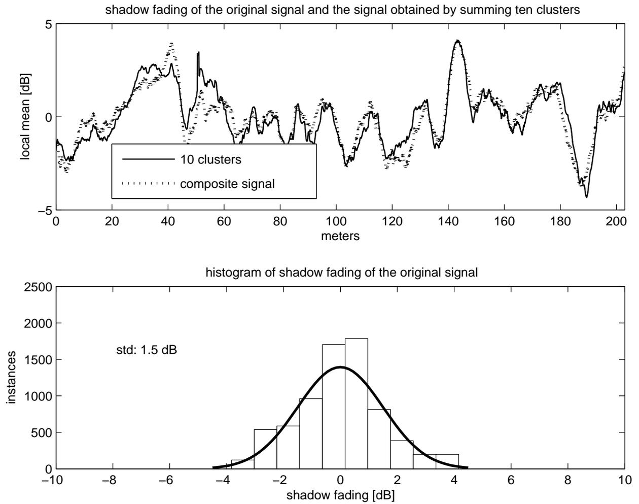
Fig. 9. Shadow fading process of the original measured signal, and signal reconstructed by summing the shadow fadings of ten clusters.
