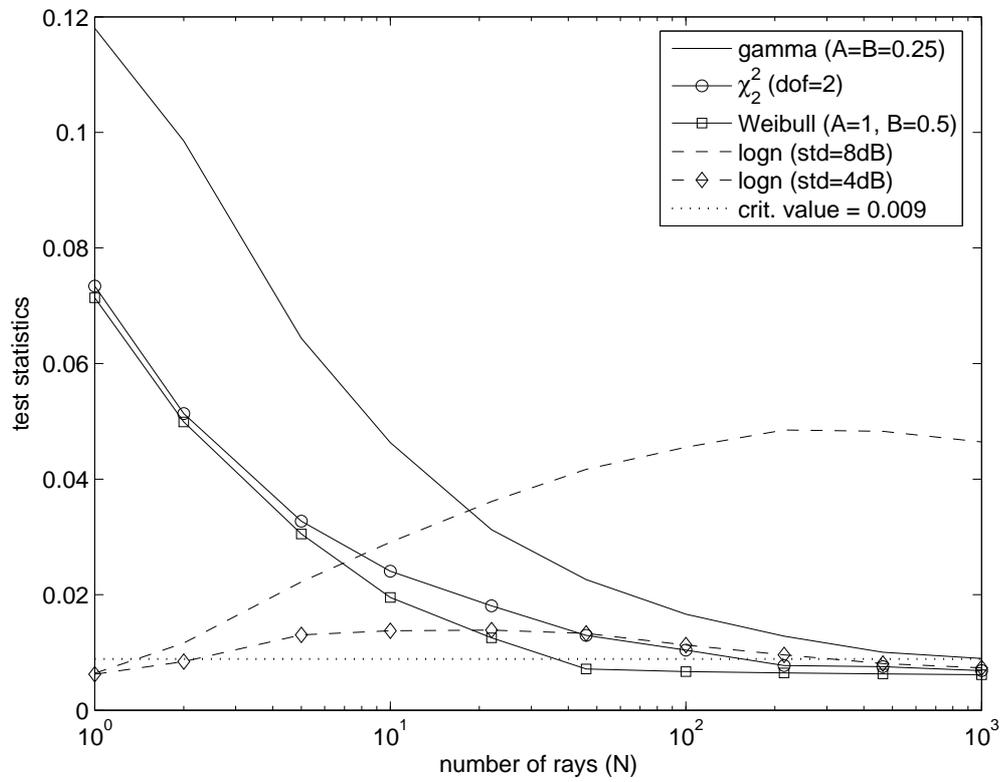
Fig. 6. Modified Kolmogorov-Smirnov hypothesis test to compare the goodness of fit of  $10 \log_{10}(\mathcal{P}_N)$  to Gaussian distribution. The critical value for 5% significance level is also shown. Small value of the test statistics indicates good fit.
