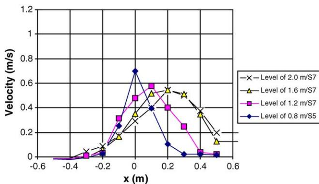
Fig. 4. Maximum velocity profiles above the induction range. X-axis is the cross section across the length of the appliance. The “S”-cross sections are across the width of the appliance. The “S6”-cross section is in the middle of the appliance.
