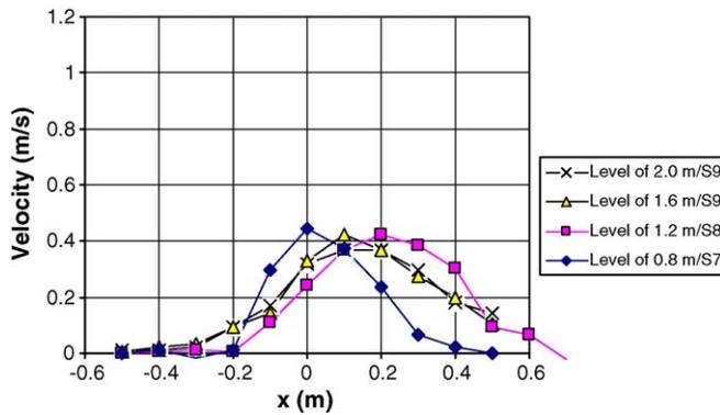
Fig. 6. Maximum velocity profiles above the fryer X-axis is the cross section across the length of the appliance. The “S”-cross sections are across the width of the appliance. The “S6”-cross section is in the middle of the appliance.
