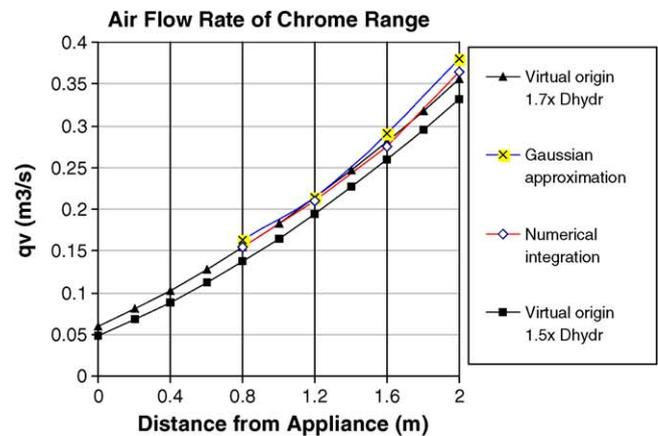
Fig. 8. Measured and calculated airflow rates of the high heat gain appliances.
