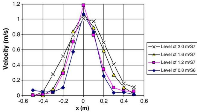
Fig. 3. Maximum velocity profiles above the gas range. X-axis is the cross section across the length of the appliance. The “S”-cross sections are across the width of the appliance. The “S6”-cross section is in the middle of the appliance.
