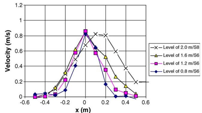
Fig. 2. Maximum velocity profiles above a chrome range. X-axis is the cross section across the length of the appliance. The “S”-cross sections are across the width of the appliance. The “S6”-cross section is in the middle of the appliance.
