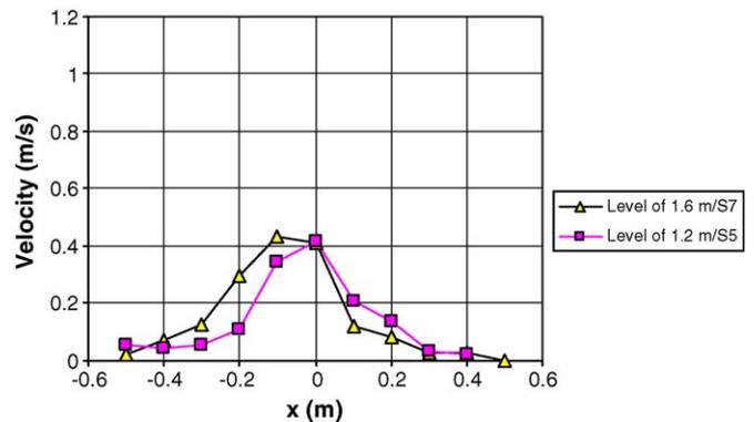
Fig. 5. Maximum velocity profiles above an induction griddle X-axis is the cross section across the length of the appliance. The “S”-cross sections are across the width of the appliance. The “S6”-cross section is in the middle of the appliance.
