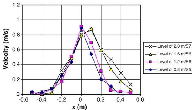
Fig. 1. Maximum velocity profiles above an iron range. X-axis is the cross section across the length of the appliance. The “S”-cross sections are across the width of the appliance. The “S6”-cross section is in the middle of the appliance.
