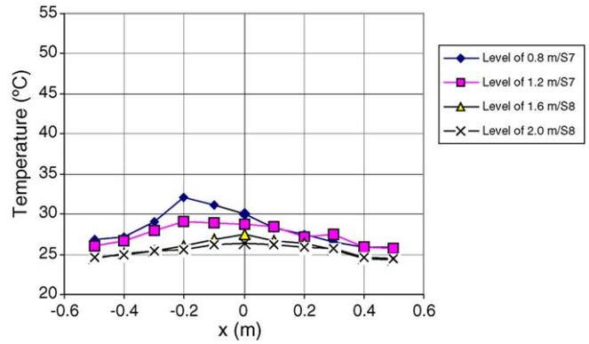
Fig. 8. Maximum temperature profiles above the induction griddle.
