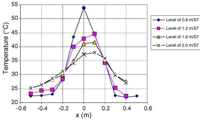
Fig. 6. Maximum temperature profiles above the gas range.
