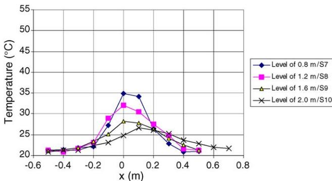
Fig. 4. Maximum temperature profiles above the chrome range.
