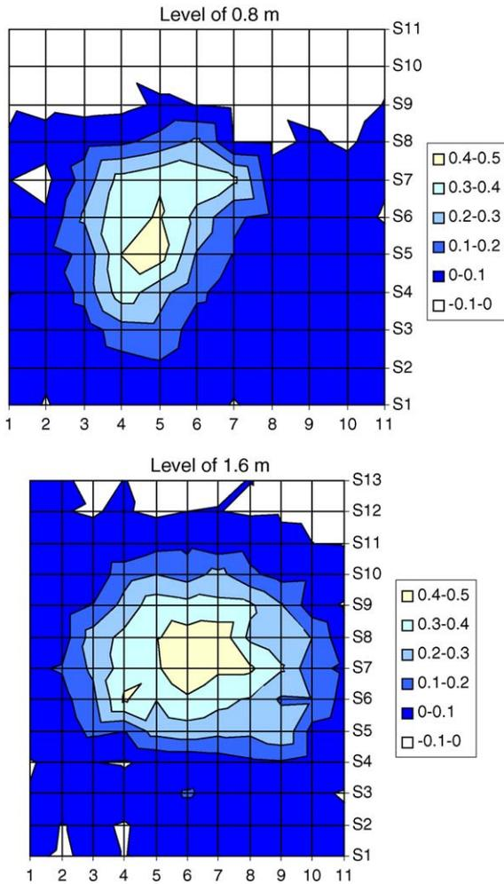
Fig. 7. Velocity distribution of the induction griddle (500 mm (W) × 800 mm (L)) at two different levels. The length of the range is accordant with Y-axis. The centre point is 6–S6 The measurement grid is 10 cm × 10 cm.
