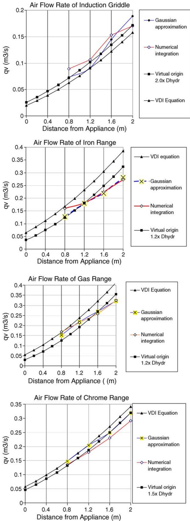
Fig. 9. Measured and calculated induced air flow rates of the plumes.
