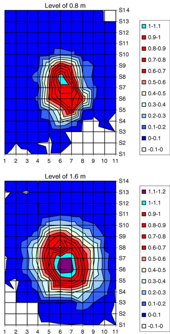
Fig. 5. Velocity distribution of the gas range (450 mm (W) × 650 mm (L)) at two different levels. The length of the range is accordant with Y-axis. The centre point is 6–S6 The measurement grid is 10 cm × 10 cm.
