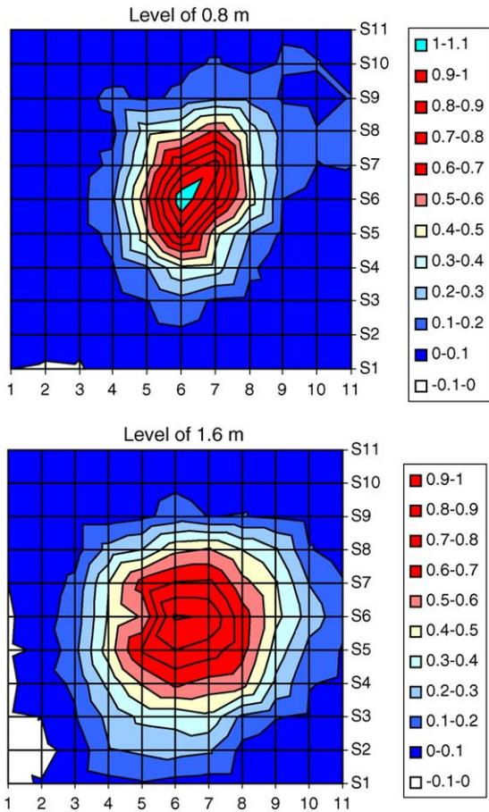
Fig. 1. Velocity distribution of the iron range (500 mm (W) × 800 mm (L)) at two different levels. The length of a range is accordant with Y-axis. The centre point is at (6–S6). The measurement grid is 10 cm × 10 cm.
