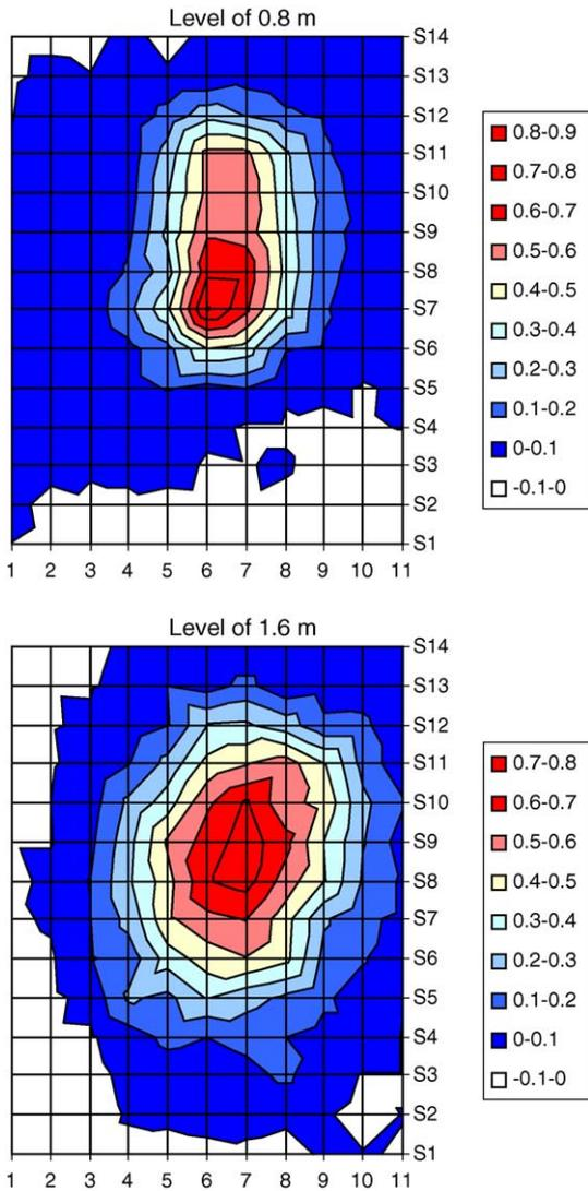
Fig. 3. Velocity distribution of the chrome range (500 mm (W) × 800 mm (L)) at two different levels. The length of a range is accordant with Y-axis. The centre point of a range is at point (6–S9). The measurement grid is 10 cm × 10 cm.
