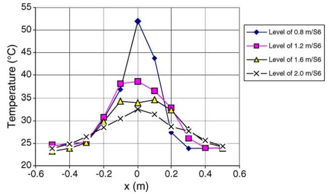
Fig. 2. Maximum temperature profiles above the iron range.
