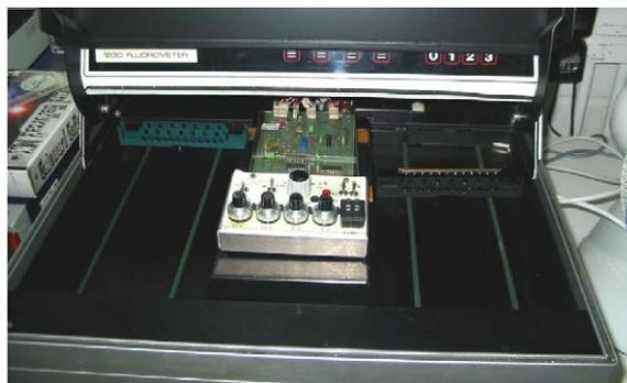
Fig. 1. Modified Arcus conveyor track also displaying the excitation electronics block added to the instrument.
