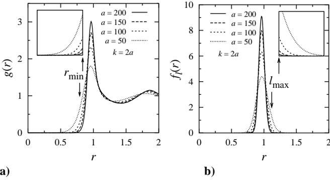
FIG. 3: **a)** Radial distribution function in the case of  $N = 32$ . The arrow shows the distance  $r_{\min}$ , and the inset the region at lengths shorter than  $r_{\min}$ . Compare with LJ models ( $r_c = 1, 2.5$ ). **b)** Bond length distribution ( $N = 32$ ). The arrow shows the location of  $l_{\max}$ , and the inset the region at values larger than  $l_{\max}$ .
