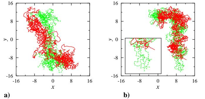
FIG. 2: The snapshots present 10 superpositions of configurations for a chain of length  $N = 256$  taken at times 100 apart. Green: times up to 500 (in DPD time units), red: times from 500 to 1000. **a)** Rouse dynamics ( $a = 25$ ,  $k = 50$ ) and **b)** reptation ( $a = 100$ ,  $k = 200$ ).
