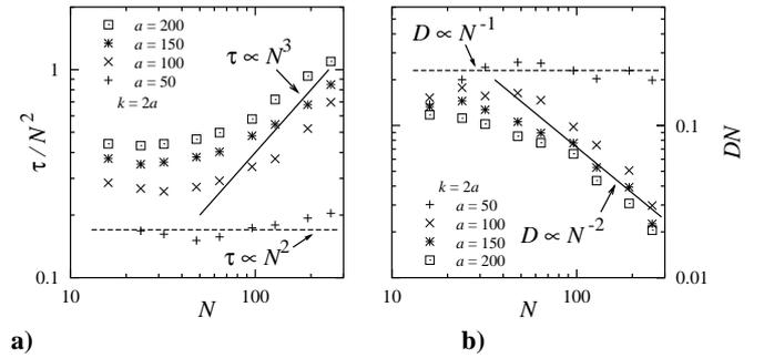
FIG. 5: **a)** Scaling of the longest relaxation time  $\tau$ . There is a crossover from Rouse scaling ( $\tau \propto N^2$ ) to reptation ( $\tau \propto N^3$ ). **b)** Similarly, the proper scaling limits are reached for the diffusion coefficient  $D$ .
