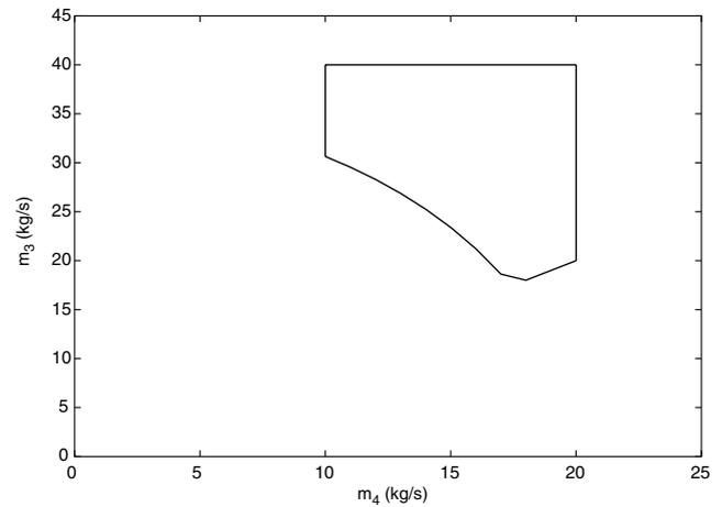
Fig. 3. Feasible region for the mass flows through the two last stages.
