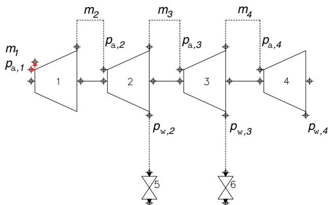
Fig. 2. Back pressure steam turbine with regulation stage and two extraction levels; The live steam temperature and pressure are 450 °C and 70 bar, respectively. The extraction pressures are 20 bar and 10 bar and the back pressure is 3 bar.
