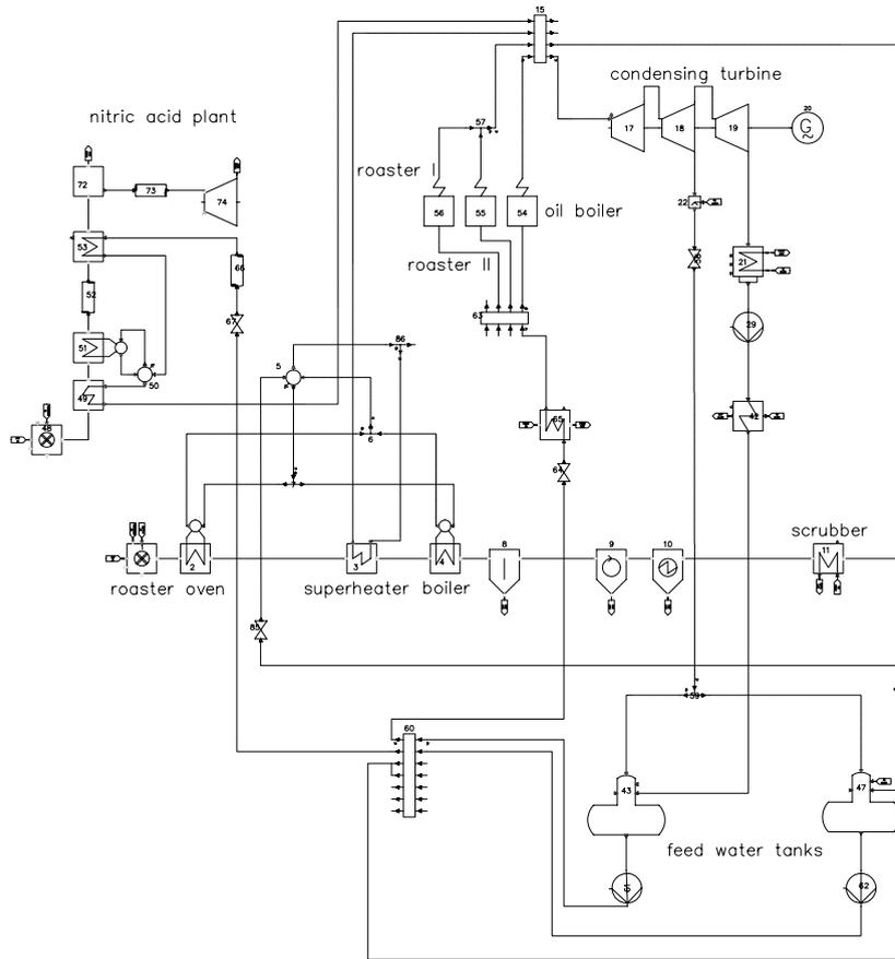
Fig. 2. First part of the Prosim simulation model of the energy system (continuous from the right in Fig. 3).
