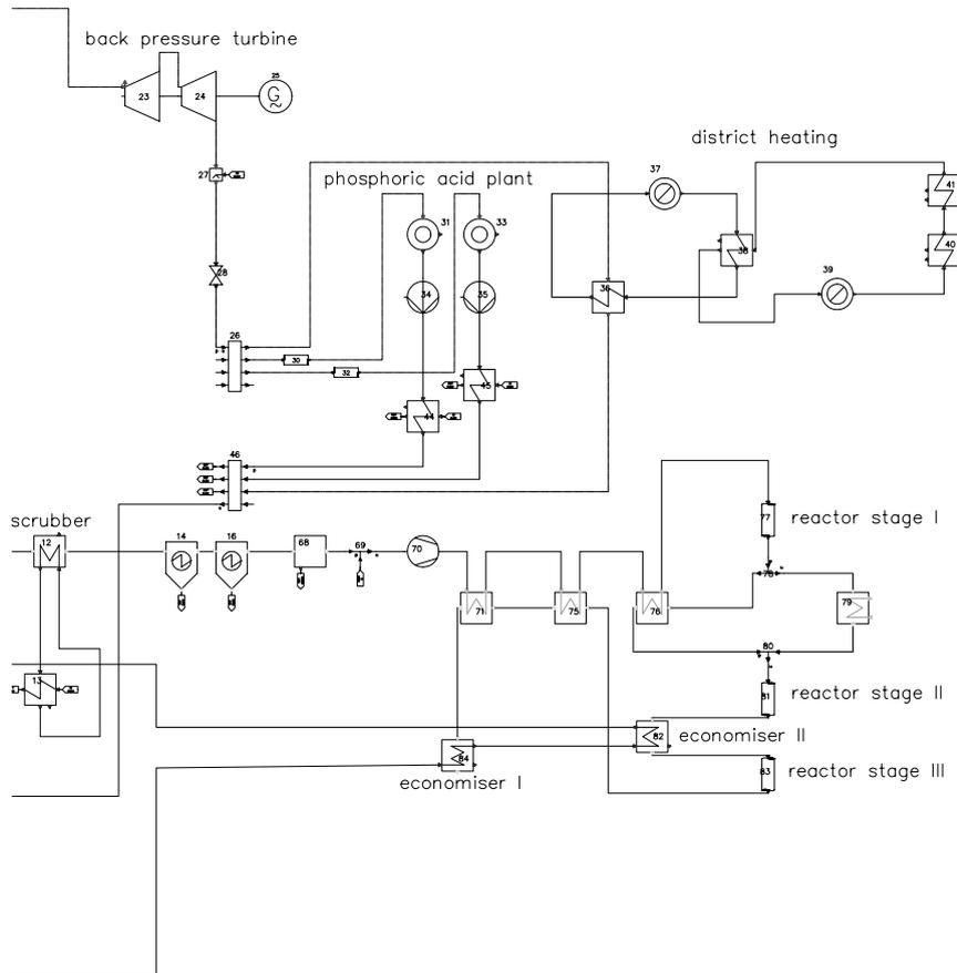
Fig. 3. Second part of the Prosim simulation model of the energy system (continued from the left from Fig. 2).
