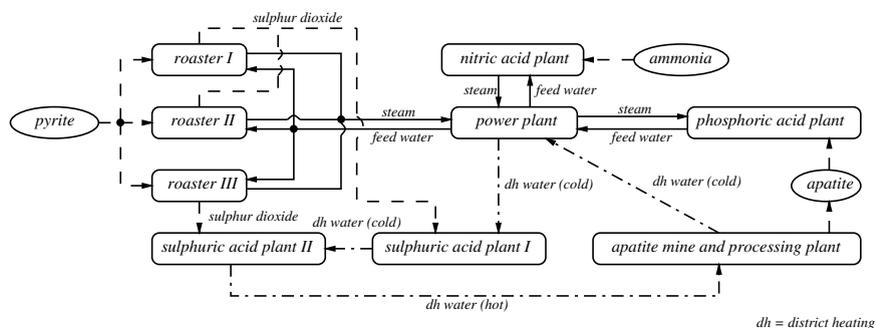
Fig. 1. The system's main energy flows except electricity.
