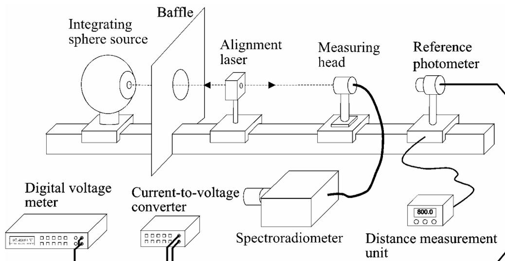
**Figure 1.** The measurement set-up for luminance and spectral radiance measurements. The alignment laser is removed from the rail when luminance or spectral radiance is measured.
