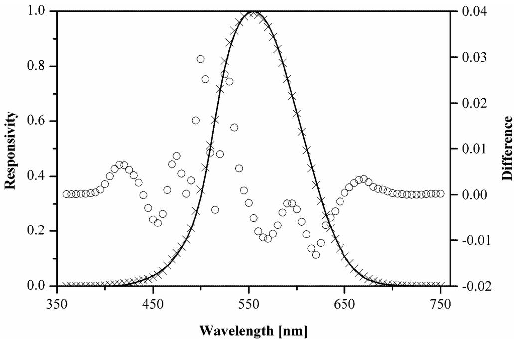
**Figure 4.** Relative spectral responsivity of the reference photometer (crosses) as compared with the  $V(\lambda)$  curve (solid line). Open circles represent the difference between the two curves.
