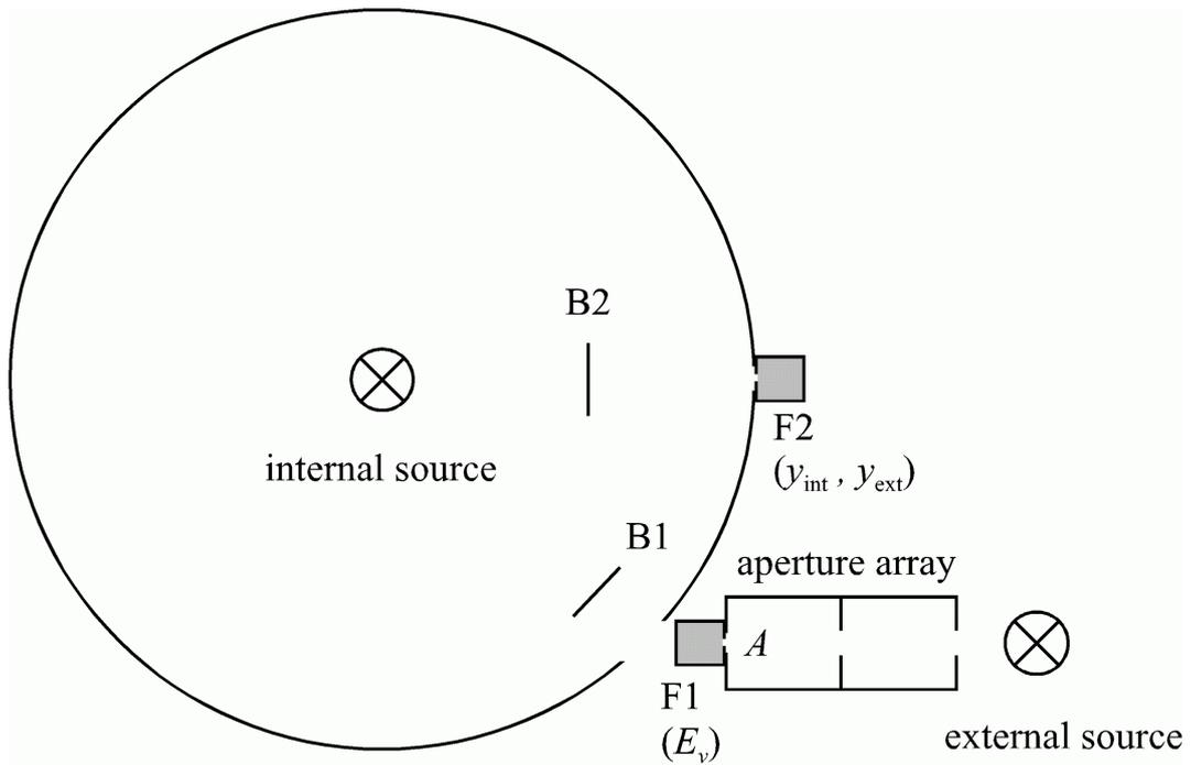
**Figure 2.** The luminous flux measurement set-up. F1 and F2 are photometers, and B1 and B2 are baffles [Publ. III].
