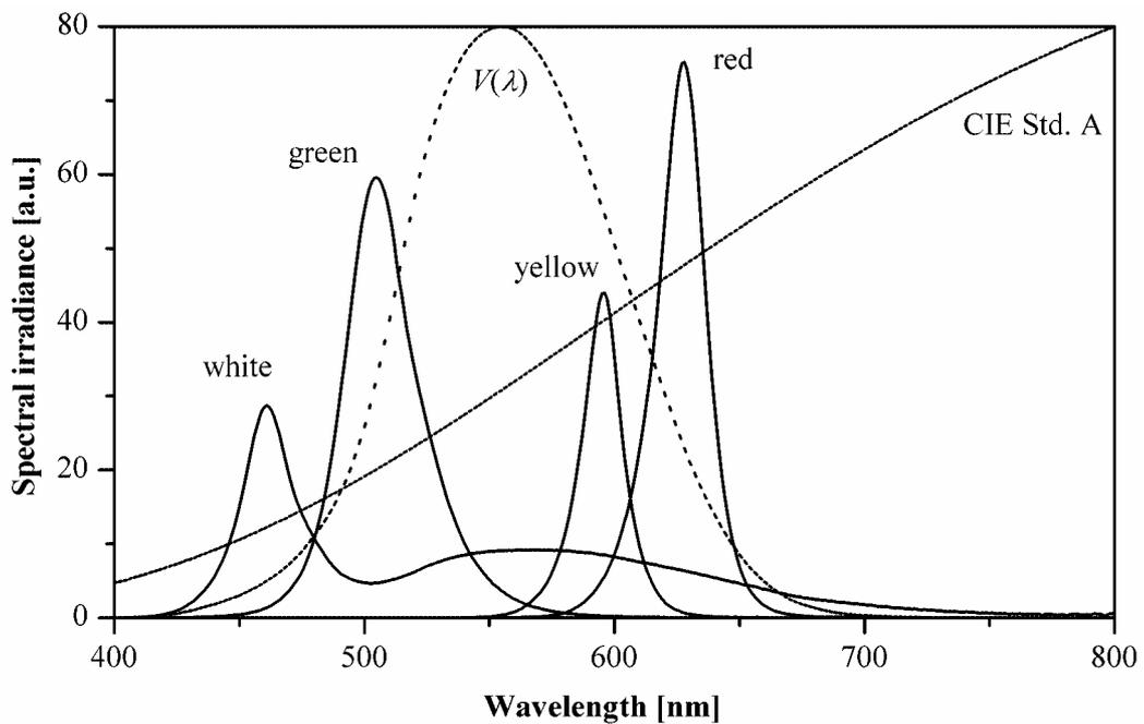
**Figure 3.** Spectral power distributions of four LEDs shown with the  $V(\lambda)$  curve and the spectrum of the CIE standard illuminant A.
