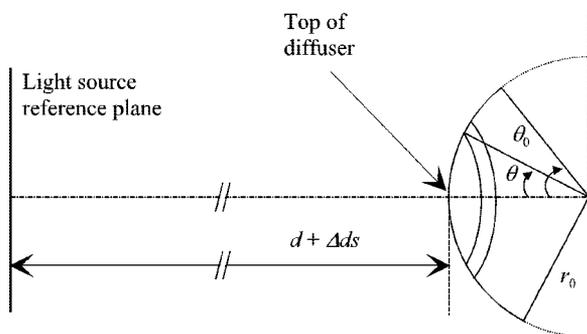
Fig. 4. Coordinate system for the calculation of the distance offset from the geometry.
