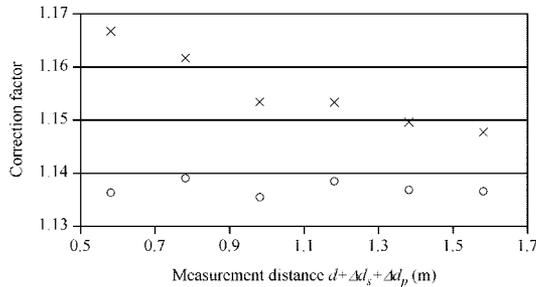
Fig. 3. Original (crosses) and new (circles) correction factors for the photometer with diffuser (b) in Fig. 1.
