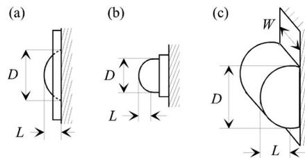
Fig. 1. Schematic drawings of the investigated diffusers. Dimensions of the diffusers in the drawings are as follows. (a)  $D = 24.3$  mm,  $L = 8.0$  mm, (b)  $D = 16.0$  mm,  $L = 7.1$  mm, (c)  $D = 30.0$  mm,  $L = 15.0$  mm,  $W = 26.1$  mm.
