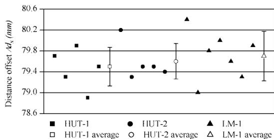
Fig. 2. Results of repeated measurements to determine the distance offset  $\Delta d_s$  of the light source with three different reference photometers. Vertical bars indicate the standard deviation of the results for each photometer.
