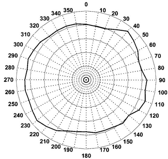
Fig. 2 The horizontal intensity distribution of the red LED lantern.
