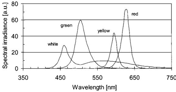
Fig. 4 Measured spectra of the LED lanterns.
