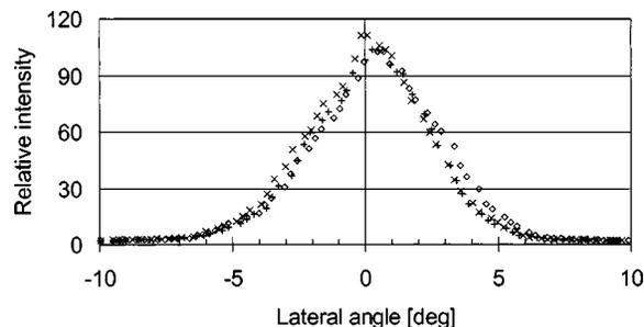
Fig. 5 Spatial illuminance intensity distribution of the red lantern with lateral angles of 0 deg (plus signs), 120 deg (crosses), and 240 deg (circles), as seen in Fig. 2.
