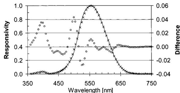
Fig. 3 Comparison of the measured spectral responsivity (crosses, normalized to 1 at 555 nm) with standardized  $V(\lambda)$  curve (solid line). Open circles represent the difference between the two curves.
