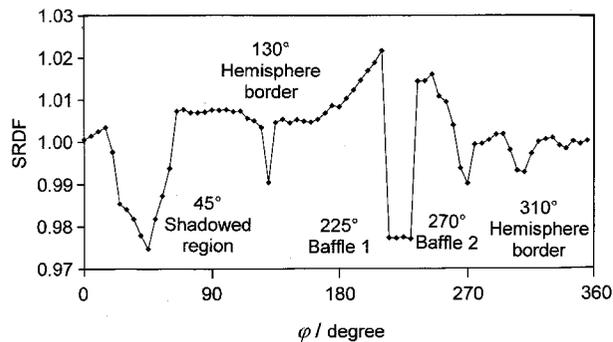
Figure 4. Equatorial SRDF of the integrating sphere.
