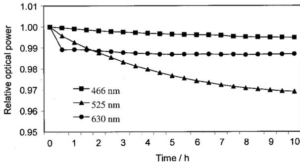
**Figure 2.** Behaviour of LED optical power as a function of time. Results of LEDs operating at wavelengths of 466 nm, 525 nm and 630 nm are presented.
