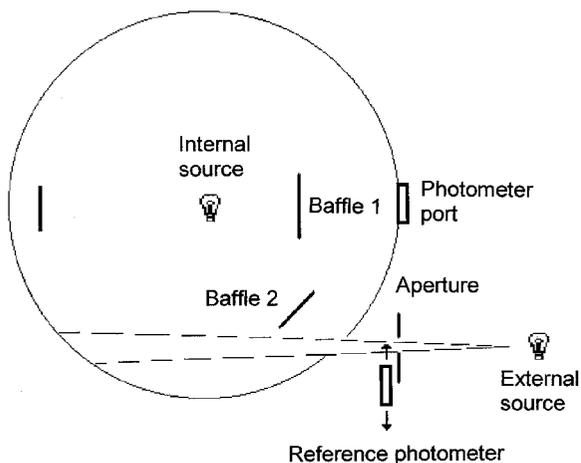
Figure 1. Apparatus used in the HUT absolute integrating-sphere method.
