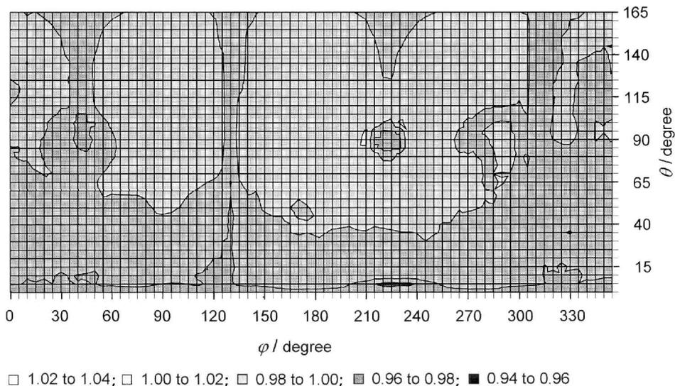
**Figure 3.** Spatial responsivity distribution function (SRDF) of the integrating sphere measured using a green LED.
