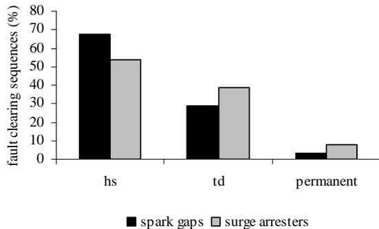
Figure 7: Shares of different fault clearing sequences.
