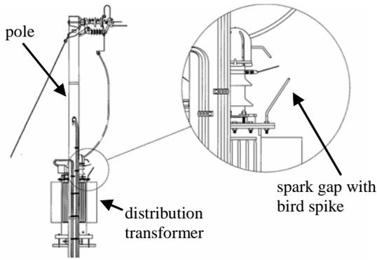
**Figure 4:** Pole-mounted distribution transformer with spark gaps.
