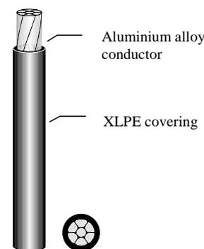
Fig. 1. Covered conductor.
