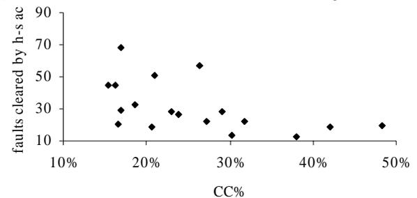
Fig. 4. The h-s fault frequency (faults/100km/year) as a function of the share of covered conductors in an overhead line feeder.
