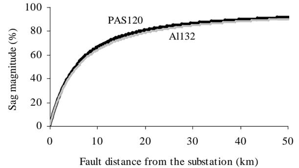
Fig. 3. Voltage sag magnitude as a function of fault distance,  $\underline{Z}_S = i 0.45 \Omega$ ,  $\underline{Z}_T = i 2.0 \Omega$ ,  $\underline{Z}_F = 0 \Omega$ .
