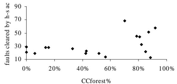
Fig. 5. The h-s fault frequency (faults/100km/year) as a function of the share of covered conductors in the forest.
