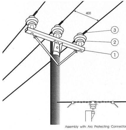
Fig. 2. Covered conductor system, pole top arrangement.
