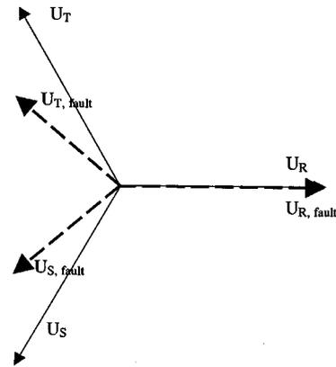
Fig. 2. Phase to neutral voltages before (solid line) and during (dashed line) a phase to phase fault.
