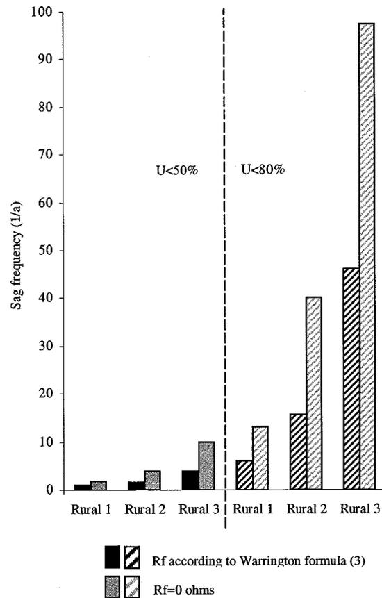
Fig. 4. Effect of fault resistance on cumulative sag frequencies.
