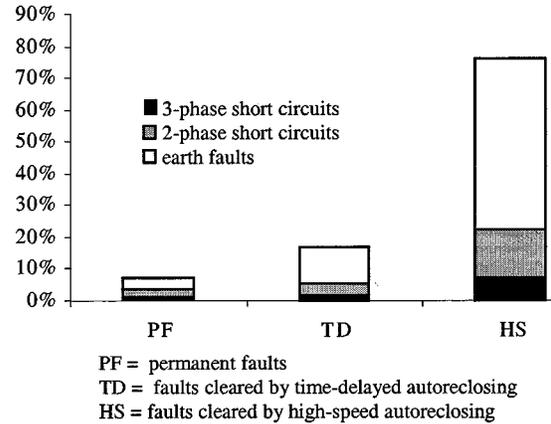
Fig. 3. Proportions of different faults in case distribution networks where autoreclosing arrangements were in use.
