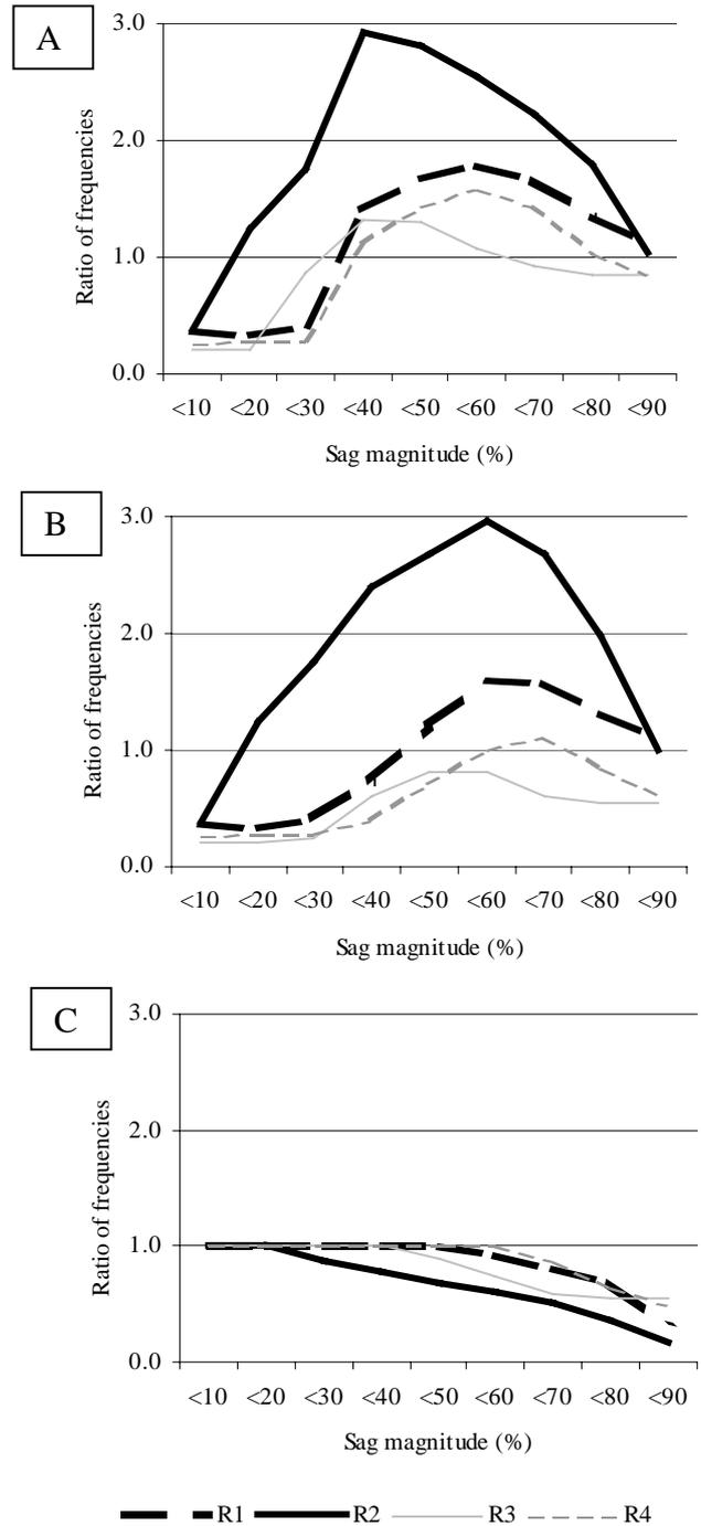
Fig. 9. The ratio of cumulative sag frequencies for mixed overhead line and underground cable networks versus purely overhead line networks.
