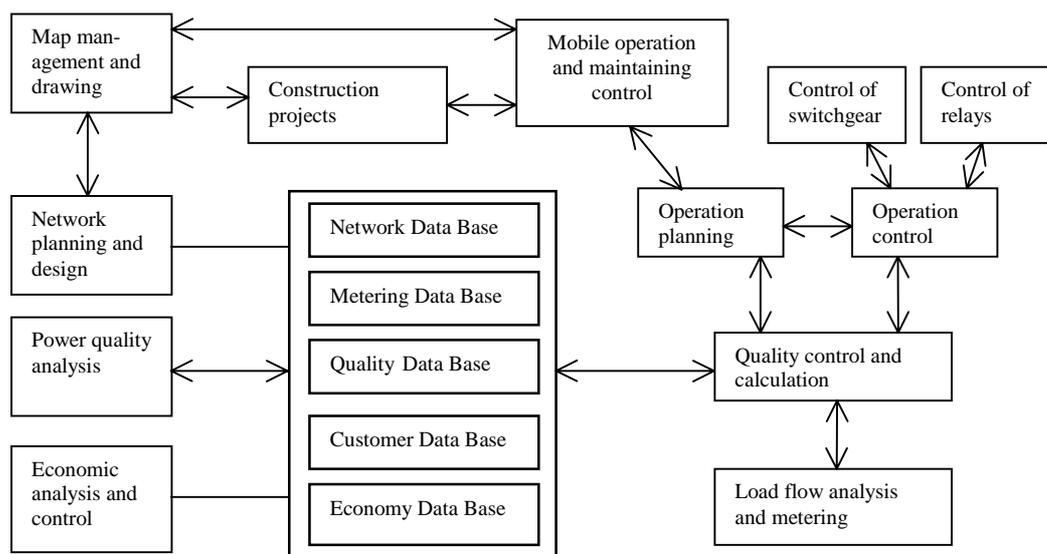
Fig. 10. The elements of distribution network information and design systems including the connections of power quality tools.
