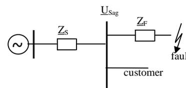
Fig. 1. Voltage divider model.
