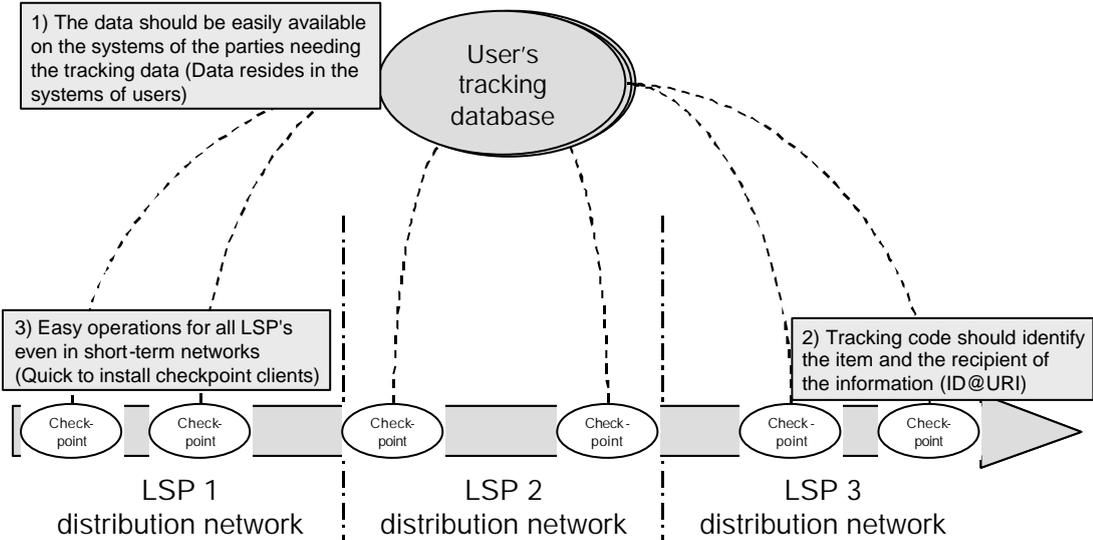
*Figure 1 The basic guidelines of forwarder independent tracking*
