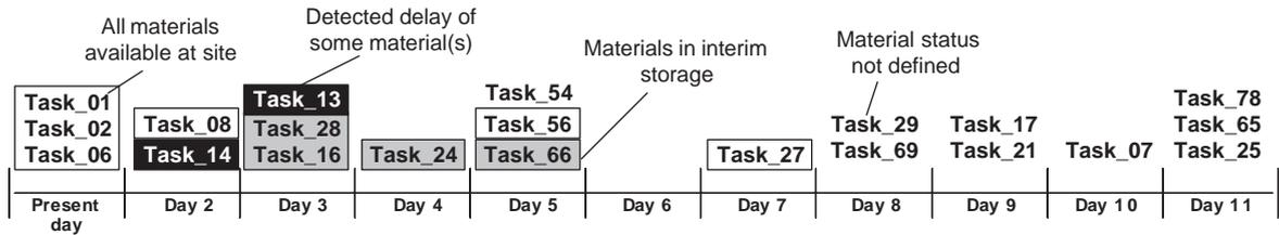
Fig. 4. Illustration of the results of materials constraint analysis.
