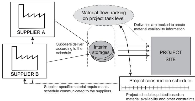
Fig. 6. An illustration of the proposed material delivery system.
