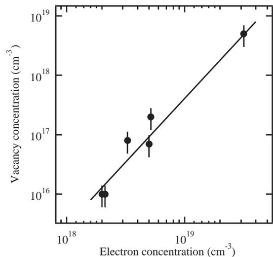
Fig. 8. In vacancy concentration vs. electron concentration. vacancy concentration is found to correlate with free electron density, as expected for compensating centers in n-type InN.
