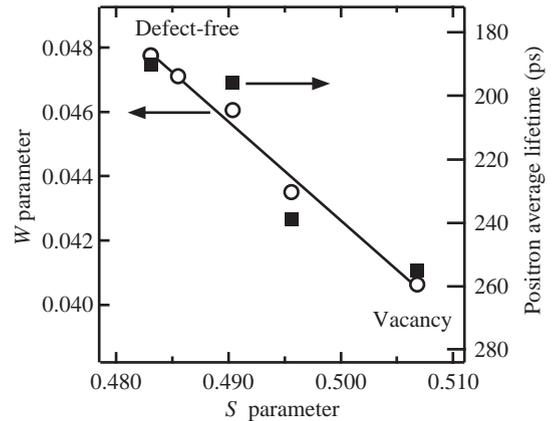
Fig. 6. The  $S$  and  $W$  parameters, and the average positron lifetime in the InN layers. The positron beam energy was kept in the range  $E = 3\text{--}7$  keV so that the layer-specific annihilation parameters were recorded. The linearity between  $S$  and  $W$ , and between  $S$  and  $\tau_{ave}$  indicates that the same vacancy is present in all layers.
