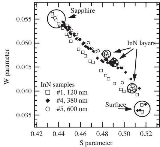
Fig. 5.  $W$  vs.  $S$  plot (positron beam energy as a running parameter) in three InN samples. The layer-specific parameters are clearly distinguished from the surface and sapphire substrate. The data points form a linear line between the sapphire and the InN layer, demonstrating no strong positron trapping effect at the interface.
