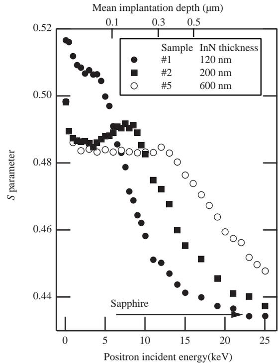
Fig. 1. The  $S$  parameter vs. positron beam energy for three different layers. The level associated with the sapphire substrate is shown with an arrow.
