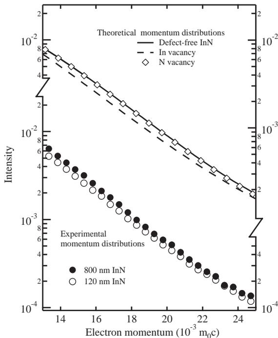
Fig. 7. The core electron momentum distributions in the InN layers. The lower panel presents the experimental results for samples #1 and #6, measured at beam energies of 2.5 and 7 keV, respectively. The upper panel shows the results of theoretical calculations for the InN lattice and for vacancies in both sublattices.
