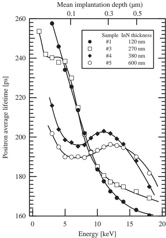
Fig. 4. The average positron lifetime  $\tau_{ave}$  vs. positron beam energy (depth scan) for four different layers. The corresponding mean implantation depth of positrons is indicated on the top axis. The lines are a guide to the eye only.
