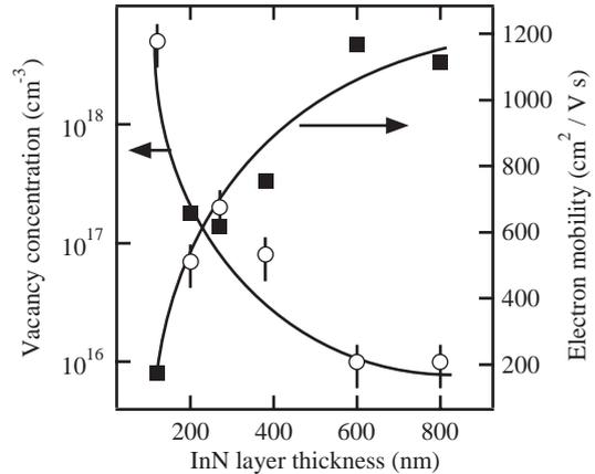
Fig. 9. Electron Hall mobility and In vacancy concentration as a function of the InN layer thickness.
