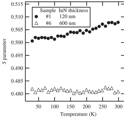
Fig. 2. The  $S$  parameter in two InN layers as a function of temperature. The positron beam energy was kept in the range  $E = 3\text{--}7$  keV so that layer specific annihilation parameters were recorded.
