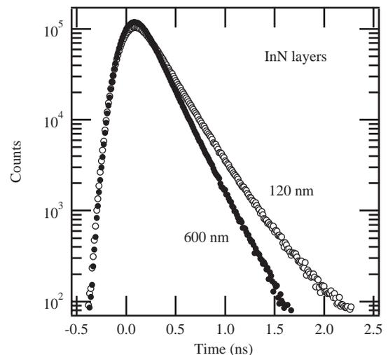
Fig. 3. Positron lifetime spectra from samples with 600 nm (black circles) and 120 nm layer (open circles) thicknesses. The spectra were measured with positron incident energies of 3 keV (120 nm layer) and 8 keV (600 nm layer). Positrons enter the sample at  $t = 0$ , and the vertical axis indicates the annihilation probability.
