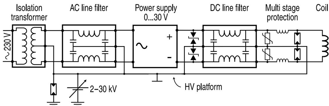
Figure 2: High voltage surge protection of power supplies of the beam. Most breakdowns are expected near the coils. Voltage spikes are guided round the power supplies to ground via the HV platform.
