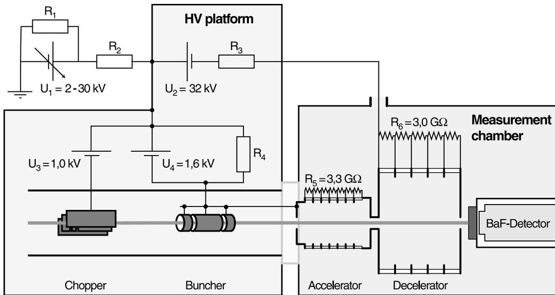
Figure 1: High voltage diagram of the lifetime beam.
