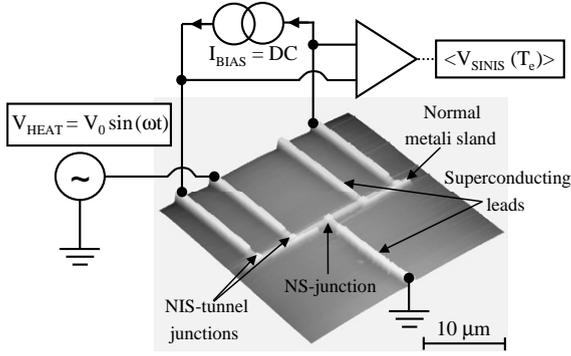
Fig. 1. An AFM image of a typical sample. The line in the middle is the Cu island and others are superconducting Al lines. Upper Al lines are connected to the Cu line with (NIS) tunnel junctions and the lower Al line is connected directly (NS junction). The sample was fabricated on a Si substrate by using electron beam lithography. The volume of the Cu island is  $\Omega = (15 \mu\text{m}) \times (450 \text{ nm}) \times (53 \text{ nm})$ .
