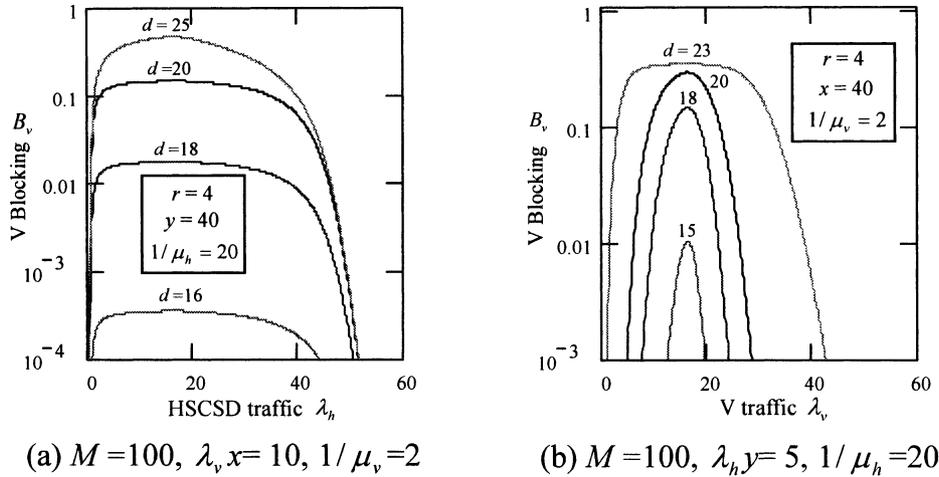
Fig. 10. V call blocking probability. (a)  $M = 100, \lambda_v x = 10$ , and  $1/\mu_v = 2$ . (b)  $M = 100, \lambda_h y = 5$ , and  $1/\mu_h = 20$ .
