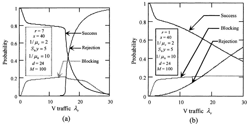
Fig. 12. Call rejection, blocking and success probabilities for V calls. Two regions are distinguished for  $r = 7$ . If  $\lambda < x e^{-1} \{1 - (1 - e^{-1})^8\}^{-1}$ , then the first region and if  $\lambda \geq x e^{-1} \{1 - (1 - e^{-1})^8\}^{-1}$ , then the next region.
