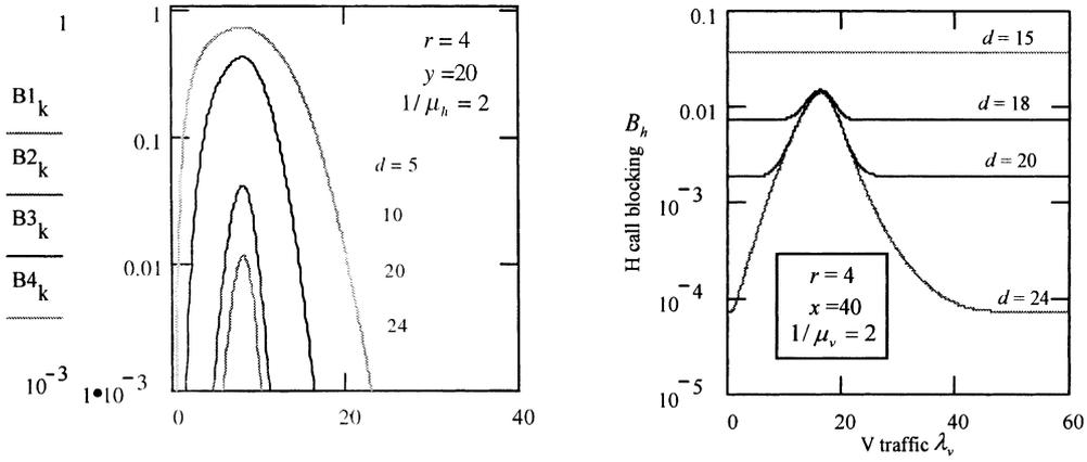
Fig. 11. HSCSD call blocking probability. (a)  $M = 100$ ,  $\lambda_v x = 3$ , and  $1/\mu_v = 2$ . (b)  $M = 100$ ,  $\lambda_h y = 2$ , and  $1/\mu_h = 5$ .
