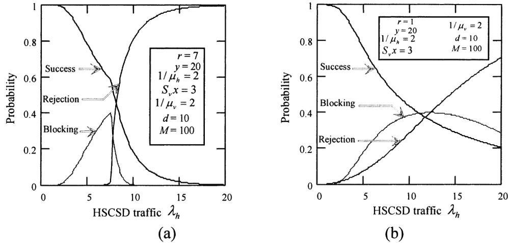
Fig. 13. Call rejection, blocking and success probabilities for H calls. Two regions are evident for  $r=7$ . If  $\lambda < xe^{-1}\{1 - (1 - e^{-1})^8\}^{-1}$ , then the first region and if  $\lambda \geq xe^{-1}\{1 - (1 - e^{-1})^8\}^{-1}$ , then the next region.
