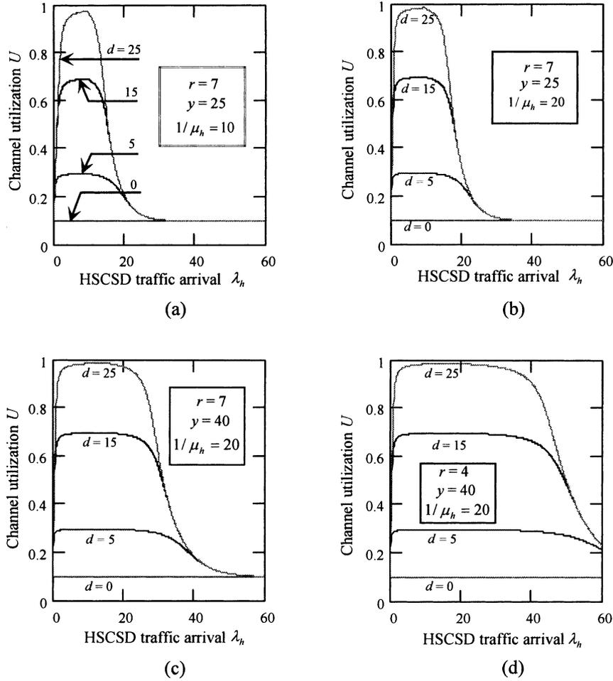
Fig. 9. Channel utilization with the variation of HSCSD traffic arrival rate.  $M = 100$ ,  $q = 4$ ,  $\lambda_v x = 10$ , and  $1/\mu_v = 2$  considered for all diagrams.
