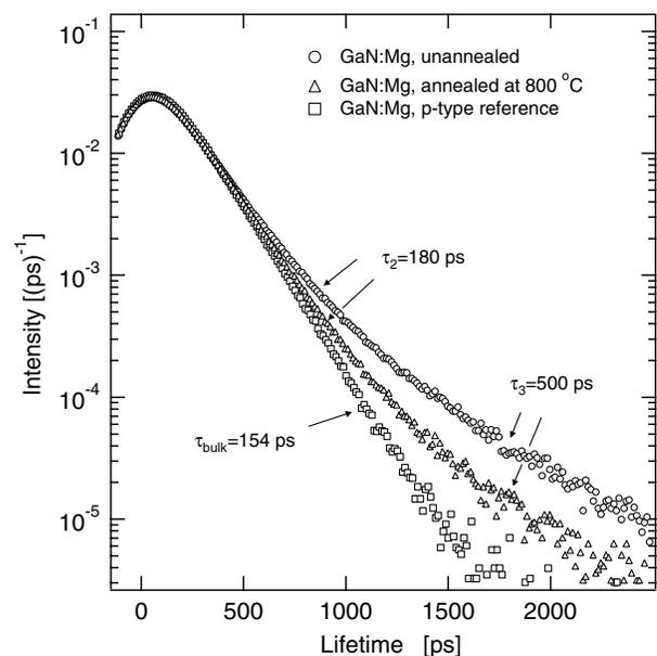
FIG. 2. The measured positron lifetime spectra in Mg-doped GaN layers, grown by MBE (reference) or by MOCVD (others). The pulsed positron beam energy was  $16\ \text{keV}$  and measuring temperature  $540\ \text{K}$ .
