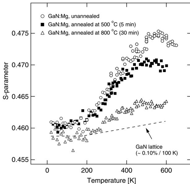
FIG. 1. The low electron-momentum parameter  $S$  as a function of temperature in MOCVD GaN samples. The dashed line represents the temperature behavior of the  $S$  parameter in the GaN lattice. Incident positron energy was  $15\ \text{keV}$ , which corresponds to a mean penetration depth of  $\approx 0.5\ \mu\text{m}$ .
