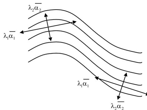
Fig. 1. A schematic illustration of the representation of anisotropy using eigenvalue decomposition. The direction of anisotropic structures is presented by two orthogonal directions confined in the matrix  $U(x) = [\bar{\alpha}_1(x), \bar{\alpha}_2(x)]$  and the strength by the corresponding eigenvalues  $\lambda_1(x), \lambda_2(x)$ .
