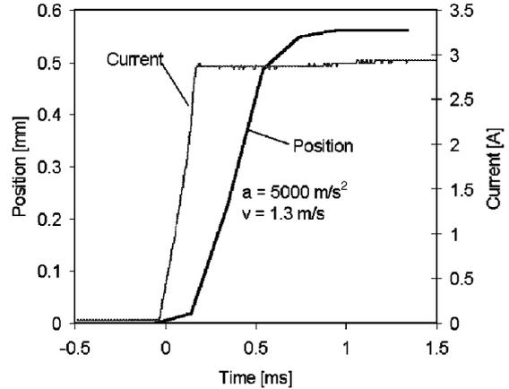
Fig. 2. Position- and current-waveform measured from the studied MSM actuator.
