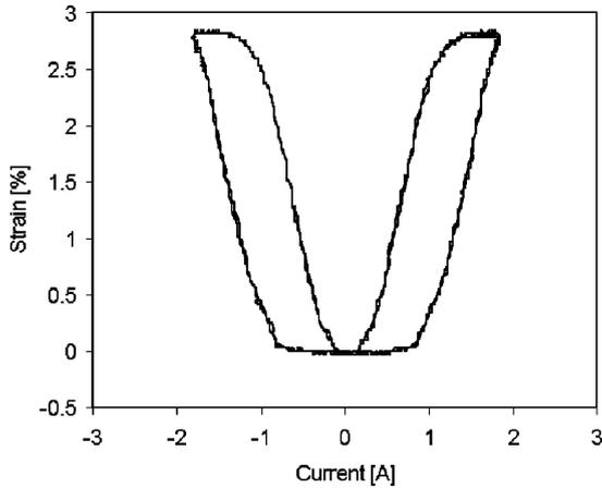
Fig. 1. Strain of an MSM element in the studied actuator, when the actuator is run with sinusoidal voltage.
