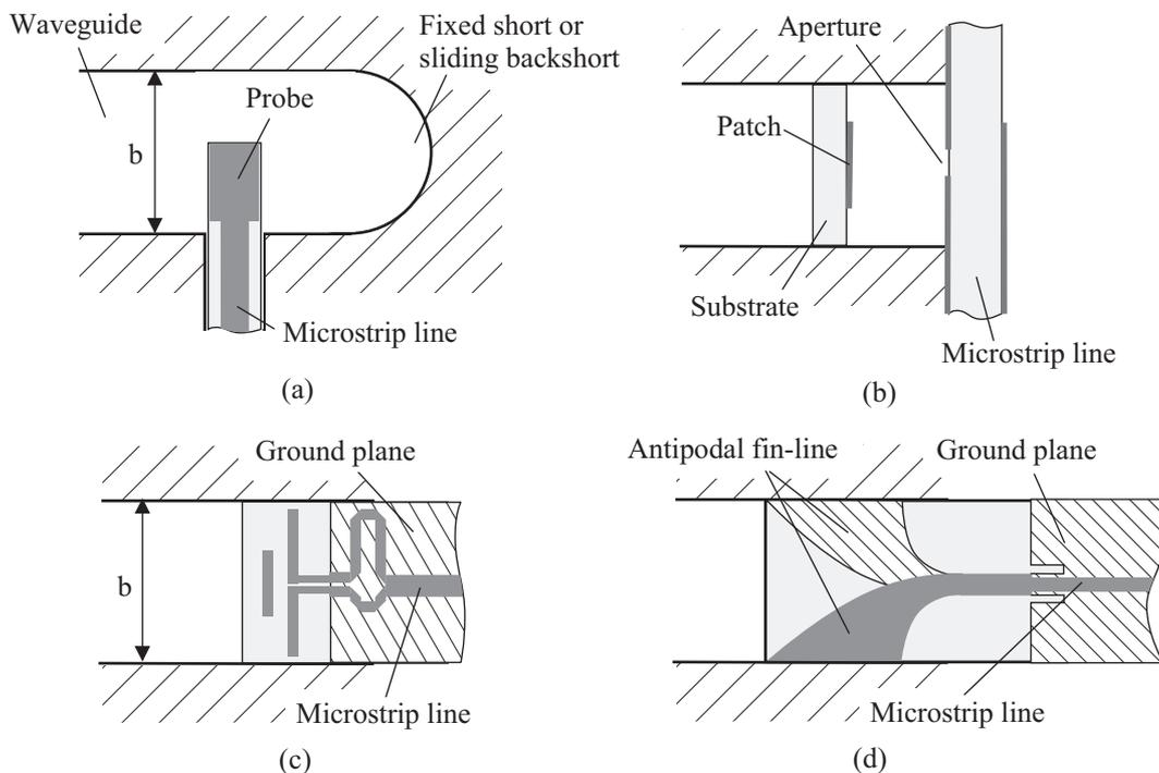
Figure 2.1. Rectangular waveguide-to-microstrip line transitions based on (a) a probe [32], (b) aperture coupling and a patch [40], (c) a quasi-Yagi antenna [42], and (d) an antipodal fin-line [43].
