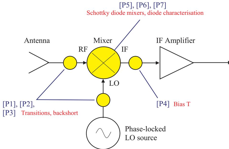
Figure 1.1. Block diagram of a typical millimetre- or submillimetre-wave receiver front-end showing (marked yellow) also the spots for components or circuits (transitions, backshort, mixers, bias T, diode characterisation), which have been developed in this thesis work, with references to publications [P1]–[P7].
