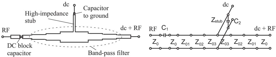
Figure 4.2. Wide-band bias T structure with six transmission line sections [74]: (a) stripline or microstrip line structure, (b) equivalent circuit (lines and stub  $\lambda/4$  in length).
