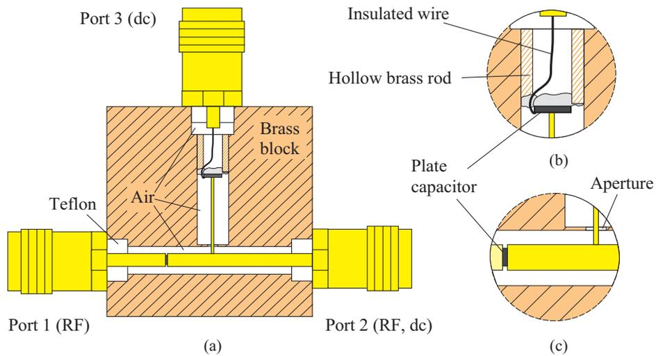
Figure 4.3. Coaxial line bias T [P4]: (a) cross-section, (b) blow-up of the RF block, (c) blow-up of the dc block and T-junction.
