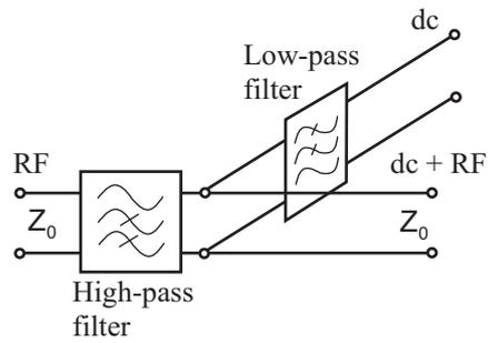
Figure 4.1. Equivalent circuit of a simple bias T.
