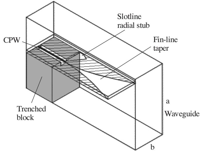
Figure 2.5. Novel CPW-to-rectangular waveguide transition using a fin-line taper and slotline radial stub [P2].
