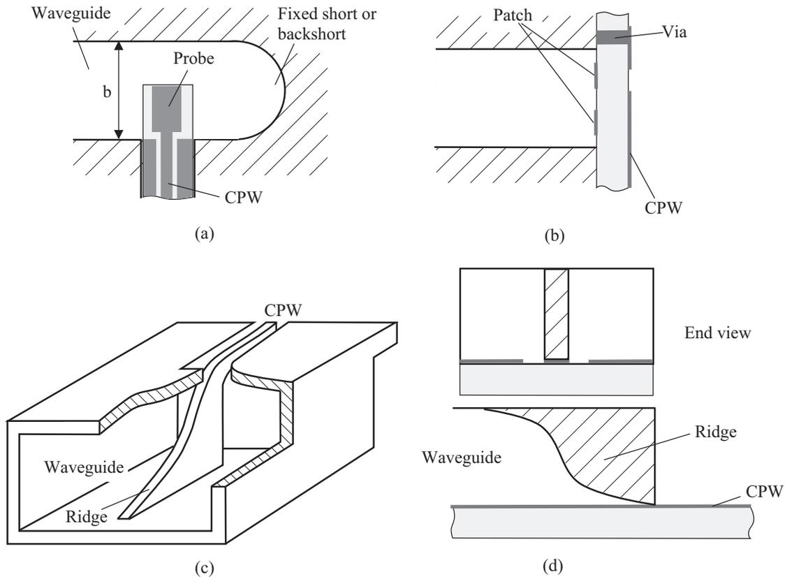
Figure 2.2. Rectangular waveguide-to-CPW transitions based on (a) a probe [45], (b) coupled patches [48], and (c), (d) ridged waveguides [49], [50].
