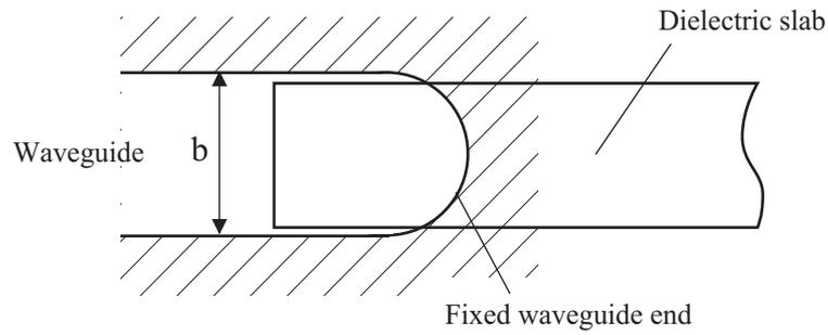
Figure 3.2. *New tunable noncontacting waveguide backshort developed in the thesis [P3]. It is based on a dielectric slab pushed into the waveguide through a hole in a fixed waveguide end. As the slab is moved the electrical length of the waveguide changes and, thus, the phase of the reflected wave changes too.*
