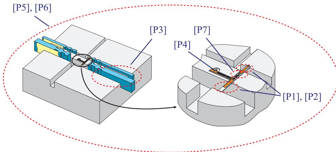
Figure 1.2. Tunable millimetre-wave waveguide mixer [P5] illustrates the spots, which have been developed in the thesis, with the original publication references [P1]–[P7]. Since this is only an illustration, all the references are not applicable to the mixer shown.
