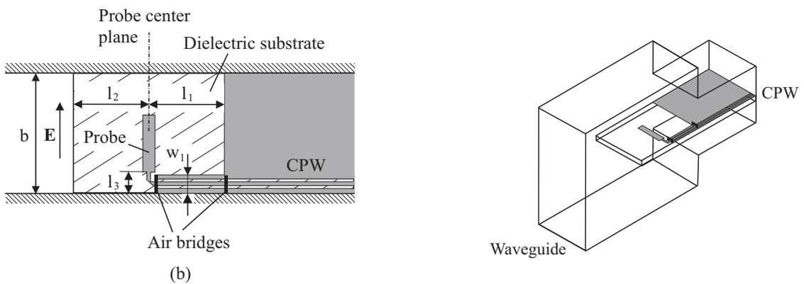
Figure 2.4. Novel rectangular waveguide-to-CPW transition based on a rectangular probe [P1]: (a) a top view and (b) an overview. An alternative waveguide housing is also shown in [P1].
