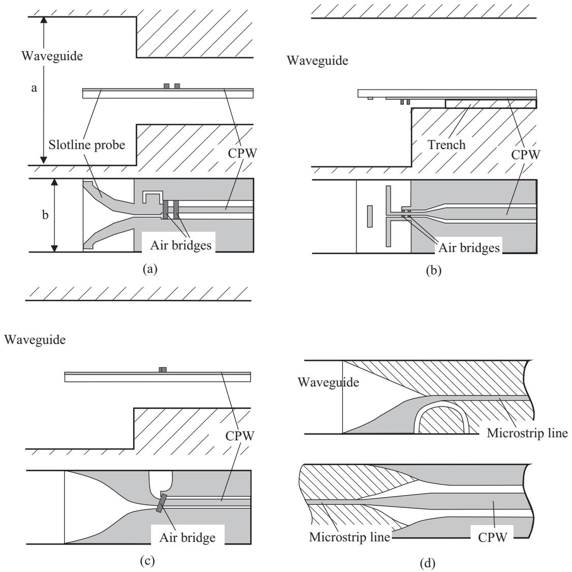
Figure 2.3. Rectangular waveguide-to-CPW transitions based on (a) a slotline probe [53], (b) a quasi-Yagi antenna [55], (c) a unilateral fin-line [56], and (d) an antipodal fin-line [57].
