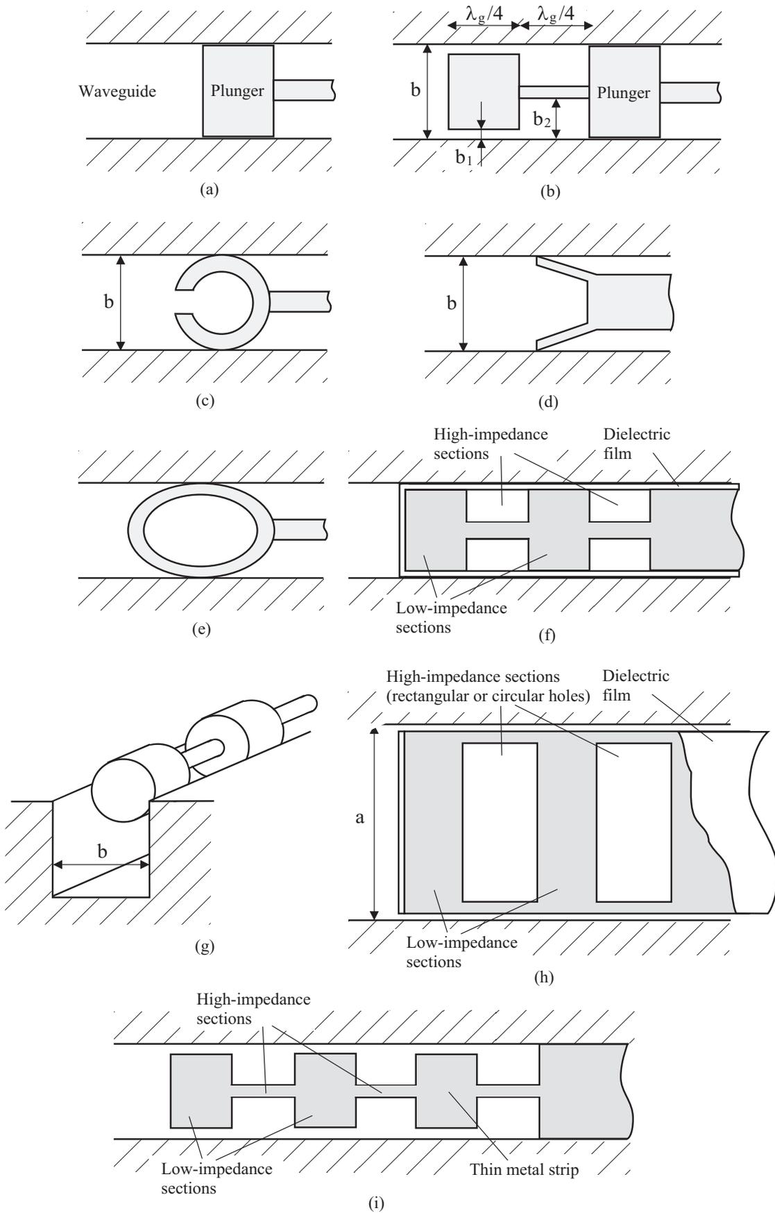
Figure 3.1. Different rectangular waveguide backshorts. (a)–(e) Contacting backshorts; (f)–(i) noncontacting backshorts. The backshort (i), with a thin metal strip in the center of the waveguide E-plane, is the only planar short circuit.
