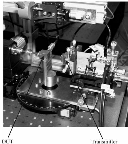
Fig. 5. Antenna measurement set-up.
