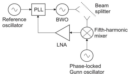
Fig. 1. Phase-locking of the backward wave oscillator (BWO) source for a submillimetre-wave antenna measurement system.
