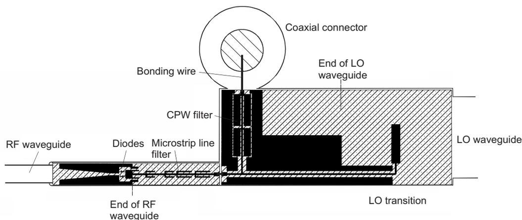
Fig. 6. Fifth-harmonic mixer circuitry comprising two 40- $\mu\text{m}$ -thick quartz substrates.
