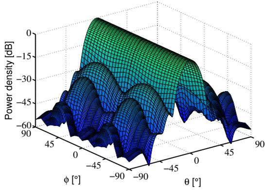
Fig. 3. Calculated co-polarised pattern of the diagonal horn antenna at 650 GHz.
