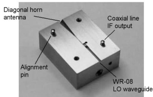
Fig. 2. Fifth-harmonic waveguide mixer block.
