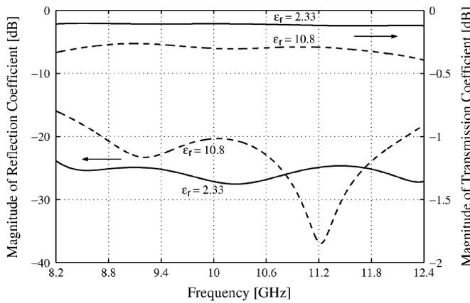
Fig. 3. Simulated magnitude of the reflection and transmission coefficient of a single  $X$ -band CPW-to-waveguide transition. Solid lines are for  $\epsilon_r = 2.33$  and dashed lines for  $\epsilon_r = 10.8$ .
