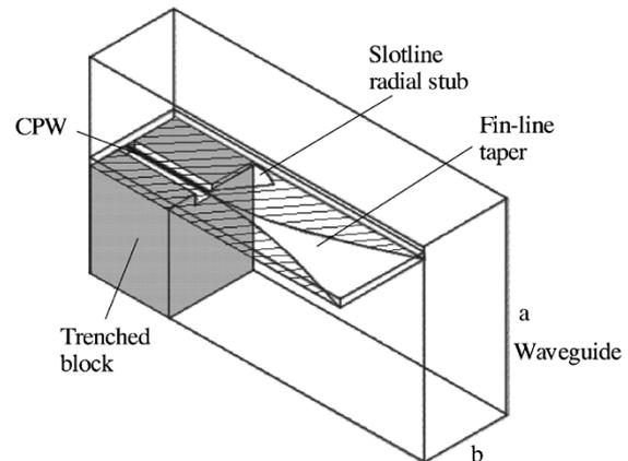
Fig. 1. Overall picture of the CPW-to-rectangular waveguide transition using a fin-line taper.
