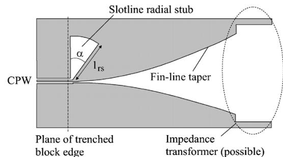
Fig. 2. Circuit layout of the waveguide-to-CPW transition using a slotline radial stub in the CPW-to-fin-line transition.
