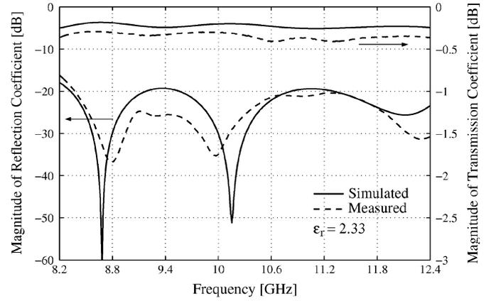
Fig. 4. Simulated and measured magnitude of the reflection and transmission coefficient of a back-to-back double  $X$ -band CPW-to-waveguide transition ( $\epsilon_r = 2.33$ ). Solid lines are for simulated and dashed lines for measured results.
