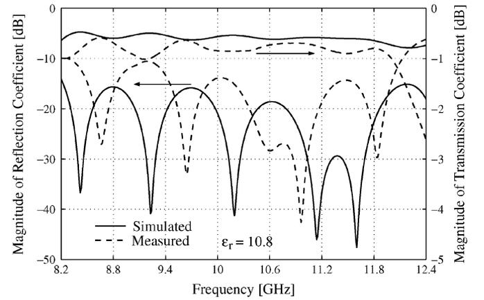
Fig. 5. Simulated and measured magnitude of the reflection and transmission coefficient of a back-to-back double  $X$ -band CPW-to-waveguide transition ( $\epsilon_r = 10.8$ ). Solid lines are for simulated and dashed lines for measured results.
