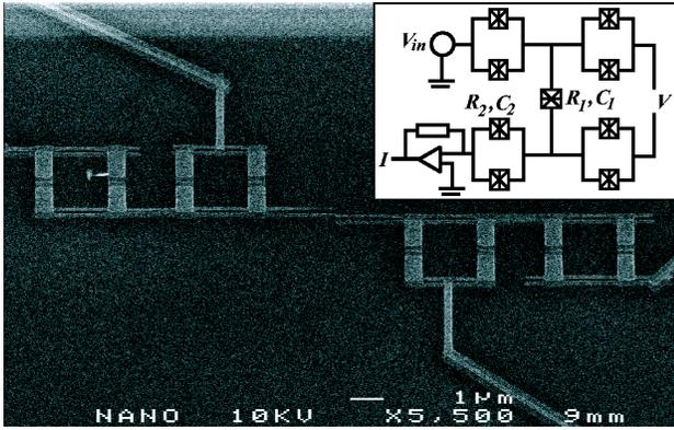
FIG. 1. SEM micrograph of a sample with four SQUID's. The probe junction has an area of  $100 \times 100 \text{ nm}^2$  and the SQUID junctions  $150 \times 550 \text{ nm}^2$ . In the samples covered in this paper, additional gate leads were available for the islands. Inset shows the schematic of the circuit in the 4-lead measurement.
