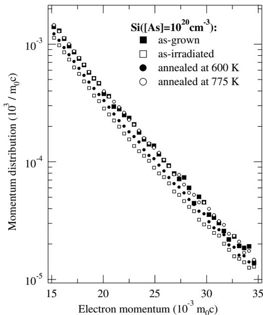
FIG. 3. Core electron momentum distribution for native (black squares) or irradiation-induced (other markers) vacancies in sample  $\text{Si}([\text{As}] = 10^{20} \text{ cm}^{-3})$ . In the as-grown Si the figure shows the decomposed spectrum where annihilations in the defect-free Si lattice have been removed [10].
