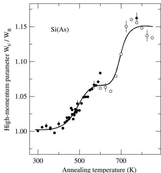
FIG. 2. Relative  $W$  parameter of the vacancy defect as a function of annealing temperature. Solid points are measured in sample Si([As] =  $10^{20} \text{ cm}^{-3}$ ) and open circles in Si([As] =  $10^{19} \text{ cm}^{-3}$ ).
