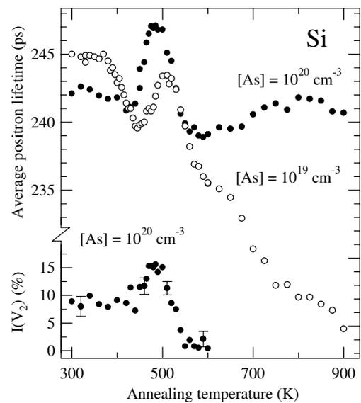
FIG. 1. Average positron lifetime and the intensity  $I_{V2}$  of the divacancy lifetime component ( $\tau_{V2} = 300$  ps) as a function of annealing temperature. All measurements were done at 300 K.  $I_{V2}$  has been determined by fixing  $\tau_{V2} = 300$  ps in the analysis of positron lifetime spectra.
