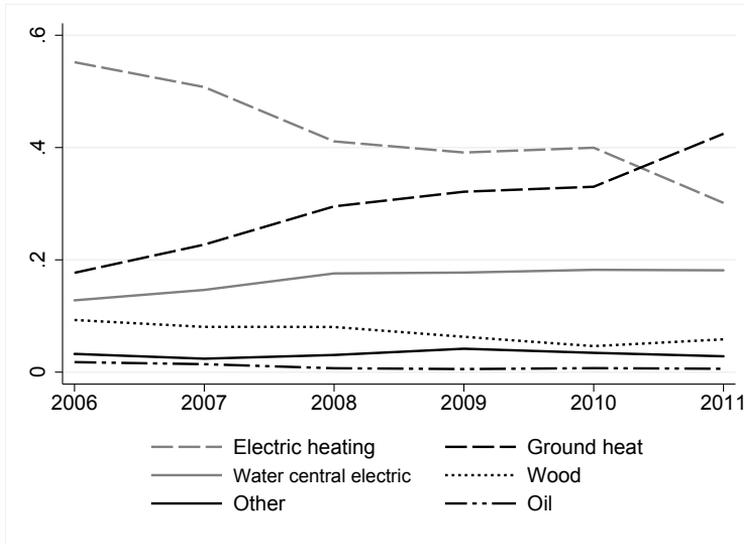
**Figure 1.** Heating technology shares in new houses.
