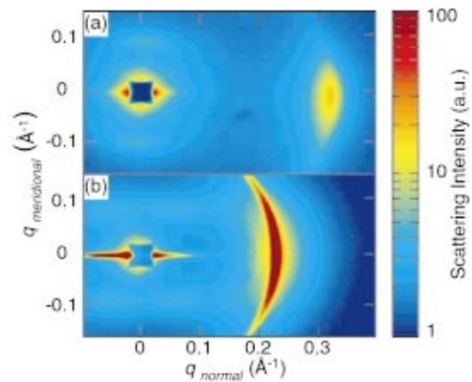
FIG. 3. (Color) Two-dimensional x-ray diffraction patterns at low angle. (a) Solid PPY(CSA)<sub>0.25</sub>(PRES)<sub>0.25</sub>. (b) Fluid PPY(CSA)<sub>0.5</sub>(OP)<sub>1.0</sub> at  $25 \text{ }^\circ\text{C}$ .
