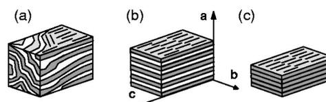
FIG. 1. (a) Self-assembled local structure. White layers denote side chains. (b) Alignment leads to macroscopically ordered structure characterized by axes **a**, **b**, and **c**. (c) Solid films due to cleavage of the side chains.
