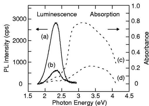
FIG. 5. The PL spectra of aligned films of PPY(CSA)<sub>0.5</sub>(HRES)<sub>0.5</sub> (solid lines) obtained with the  $c$  axis in vertical orientation: Both the excitation light ( $\lambda=370$  nm) and the PL are polarized (a) parallel and (b) perpendicular to the  $c$  axis. The PA curves (dashed lines) measured with polarized light. (c) The  $c$  axis parallel to the polarization vector of the probe light. (d) Their mutual perpendicular orientation.
