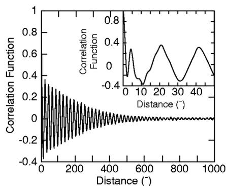
FIG. 4. The normalized  $\gamma(0)=1$  correlation function  $\gamma(r) = \int q^{-2} I(q) \cos(qr) dq$  normal to lamellae of PPY(CSA)<sub>0.5</sub>(HRES)<sub>0.5</sub> using  $q$  range between 0–2.2 Å<sup>-1</sup>. The maximum at 21 Å corresponds to  $d_{100}$  and the peak at 4 Å corresponds to the flat halo between 1–1.5 Å<sup>-1</sup> related to internal structure along the  $a$  axis.  $\alpha=\beta=\gamma=90^\circ$ ,  $a=20.06$  Å,  $b=6.89$  Å, and  $c=8.40$  Å.
