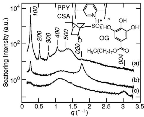
FIG. 2. X-ray diffraction curves of aligned PPY(CSA)<sub>0.5</sub>(OG)<sub>0.5</sub> in three directions: (a) Normal i.e., equatorial out-of-plane, a. (b) Equatorial, i.e., equatorial in-plane, b. (c) Meridional, c.
