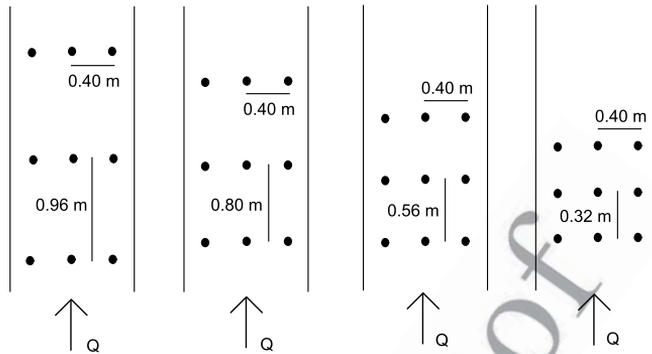
**Figure 2.** Measured spruce patterns in the flume experiments at HUT Laboratory of Water Resources.
