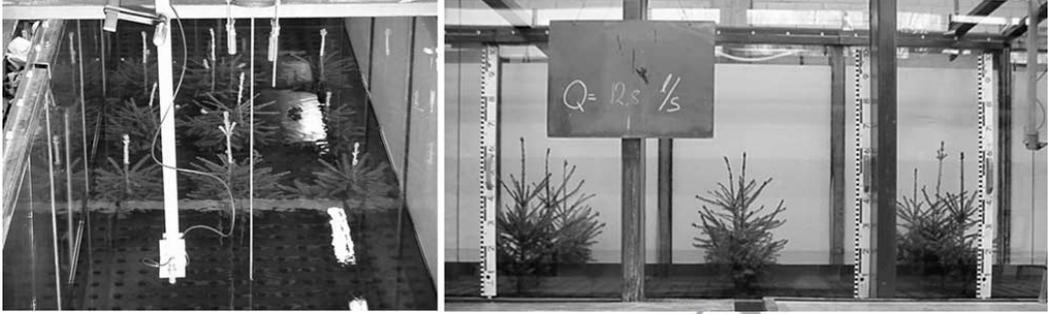
**Figure 3.** The laboratory flume experiments: (left)  $a_x = 0.56$  m,  $a_y = 0.40$  m,  $Q = 0.059$  m<sup>3</sup>/s, and  $h_{av} = 0.495$  m, from above, looking upstream; (right)  $a_x = 0.96$  m,  $a_y = 0.40$  m,  $Q = 0.0128$  m<sup>3</sup>/s, and  $h_{av} = 0.132$  m, flow from left to right.
