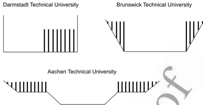
**Figure 1.** The laboratory studies on partly vegetated channels carried out in German universities in 1980s: Partly vegetated rectangular channel [Nuding, 1991], trapezoidal channel with bank vegetation [Mertens, 1989], and double-trapezoidal channel with floodplain vegetation [Pasche, 1984]
