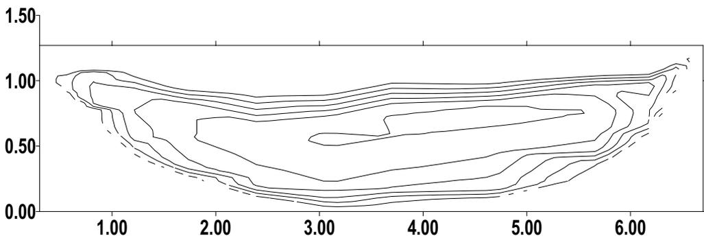
Figure 5. Example of measured velocity distribution in ice-covered channel with maximum velocity of 0.26 m/s and mean velocity 0.19 m/s. Width and height in meters.
