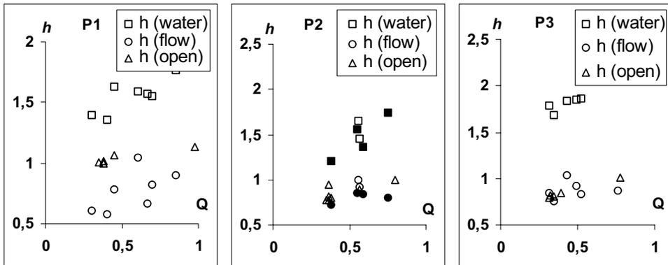
Figure 3. Water depths (i.e. the level where water rises in hole) and flow depths in winter and depths in summer as function of discharge  $Q$  ( $\text{m}^3/\text{s}$ ) in River Pääntäeenjoki (in P2 filled circles and squares after engineering works).
