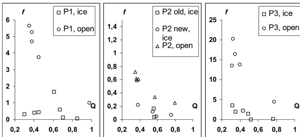
Figure 4. Darcy-Weisbach  $f$  as function of discharge  $Q$  ( $\text{m}^3/\text{s}$ ) in River Pääntäeenjoki. Results with and without ice cover are compared.
