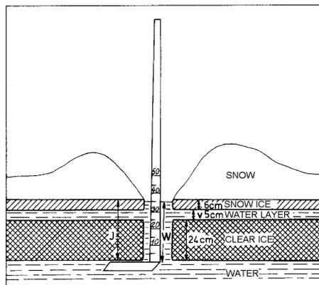
Figure 1. Measurement of ice thickness [3]
