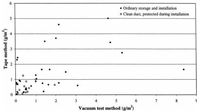
Fig. 1 A scatter plot of the data obtained using the tape and the vacuum test method (n=45)
