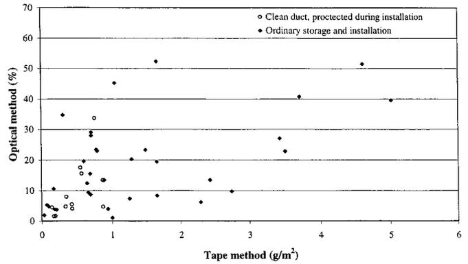
Fig. 2 A scatter plot of the data obtained using the optical and the tape method (n=45)
