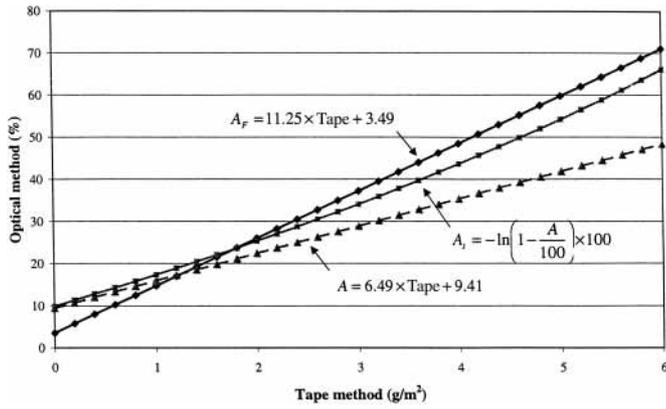
Fig. 3 Result of tape method ( $\text{g}/\text{m}^2$ ) and calculated cleanliness level of optical method (%) using equations 1–3
