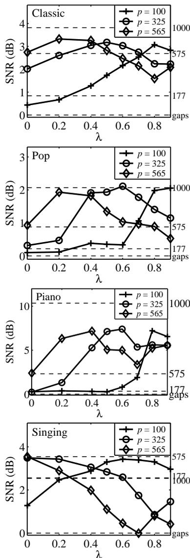
Figure 5: Average SNR of the interpolated signals under several parameter setups. Solid lines are the SNR of the restored signals as function of  $\lambda$ , for the indicated model orders. Dashed lines show the SNR of the signals when restored via the conventional method with the indicated model orders (at the end of the line on the right). The SNR of the corrupted signal is also shown (gaps).
