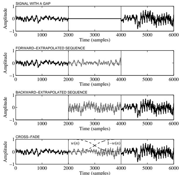
Figure 2: Steps of the interpolation scheme. The reconstructed sequence is obtained by summing the windowed ( $\alpha = 3$ ) forward- and backward-extrapolated sequences within the gap (delimited between the vertical lines).
