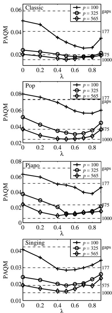
Figure 6: PAQMs of the restored signals processed under several parameter setups. Solid lines are the PAQM of the restored signals as function of  $\lambda$ , for the indicated model orders. Dashed lines are the PAQM of the signals restored via the conventional method with the indicated model orders (at the end of the line on the right). The PAQM of the corrupted signal is also shown (gaps).
