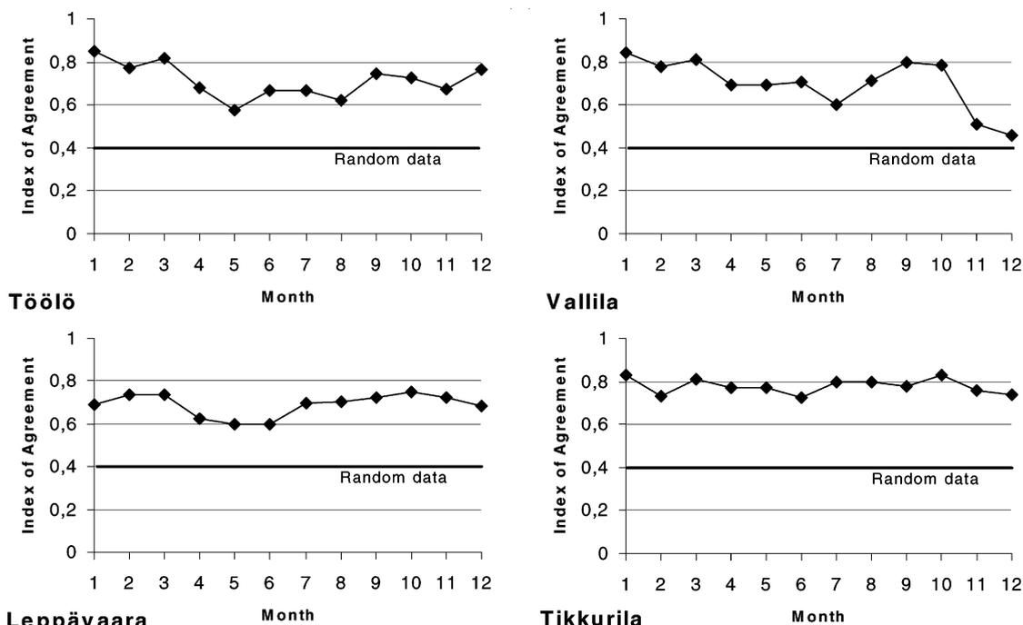
Fig. 6. a–b The index of agreement for the predicted and measured NO<sub>2</sub> concentrations at four measurement stations in Helsinki metropolitan area in 1993.
