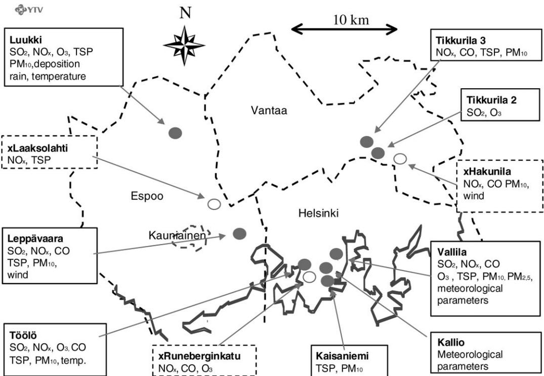
Fig. 1. The urban air quality monitoring network in Helsinki metropolitan area in 1997. The legends show the name of the station and the pollutants, which are measured continuously. The open circles correspond to the so-called ‘mobile’ stations, which are re-located each calendar year. The other stations are permanently located.
