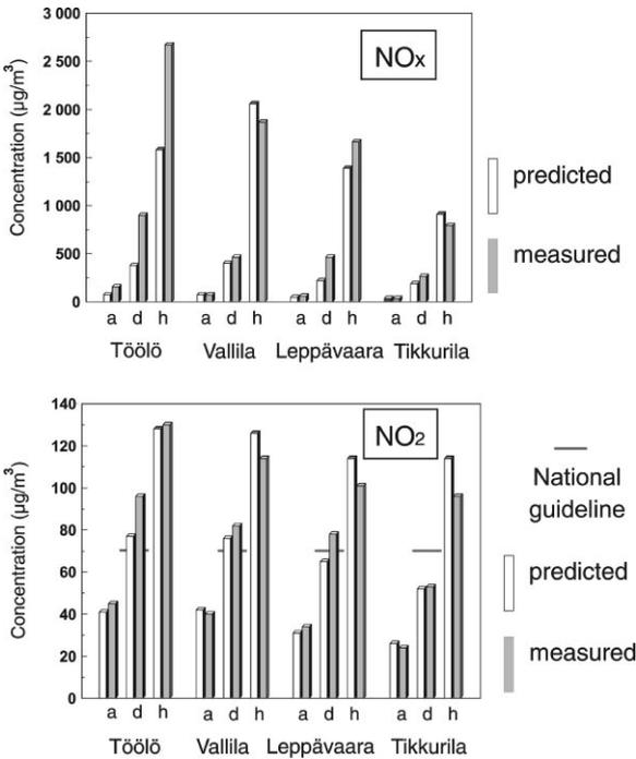
Fig. 5. a and b The predicted and measured yearly mean concentrations (denoted by a) and the statistical concentration parameters, comparable to the national guidelines for the daily (d) and hourly (h) concentrations, for NO<sub>x</sub> and NO<sub>2</sub> in the Helsinki metropolitan area in 1993.
