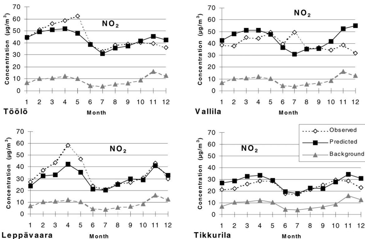
Fig. 3. a–d The predicted and measured monthly averages of NO<sub>2</sub> concentration (µg m<sup>-3</sup>) at the four monitoring stations considered, together with the regional background concentrations in 1993.
