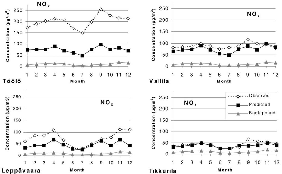
Fig. 2. a–d The predicted and measured monthly averages of the  $\text{NO}_x$  concentration ( $\mu\text{g m}^{-3}$ ) at the four monitoring stations considered, together with the regional background concentrations in 1993.
