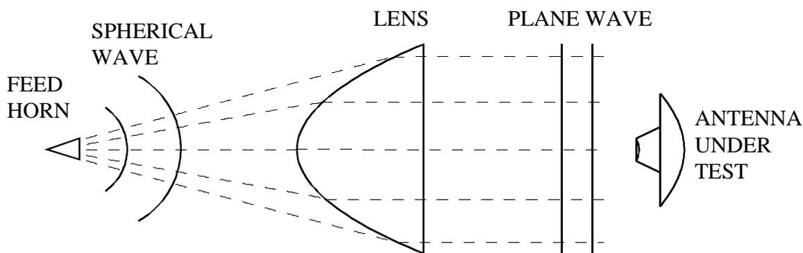
Figure 2.4: Lens type of a CATR.
