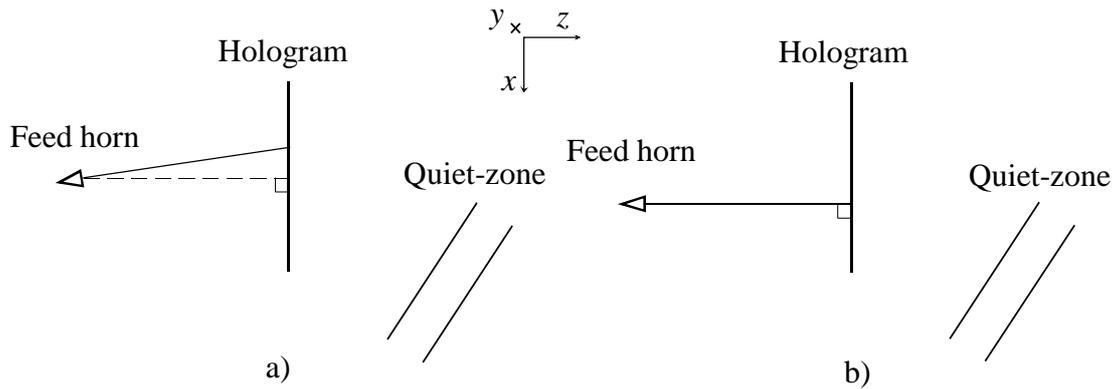
Figure 4.1: a) Rotation of the feed horn and b) offset of the feed horn.
