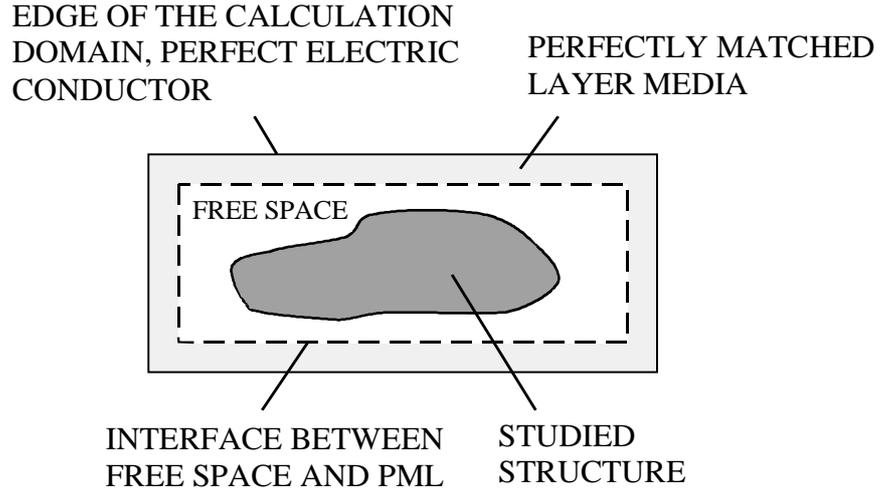
Figure 3.1: Two-dimensional calculation domain with PML absorbing boundaries.
