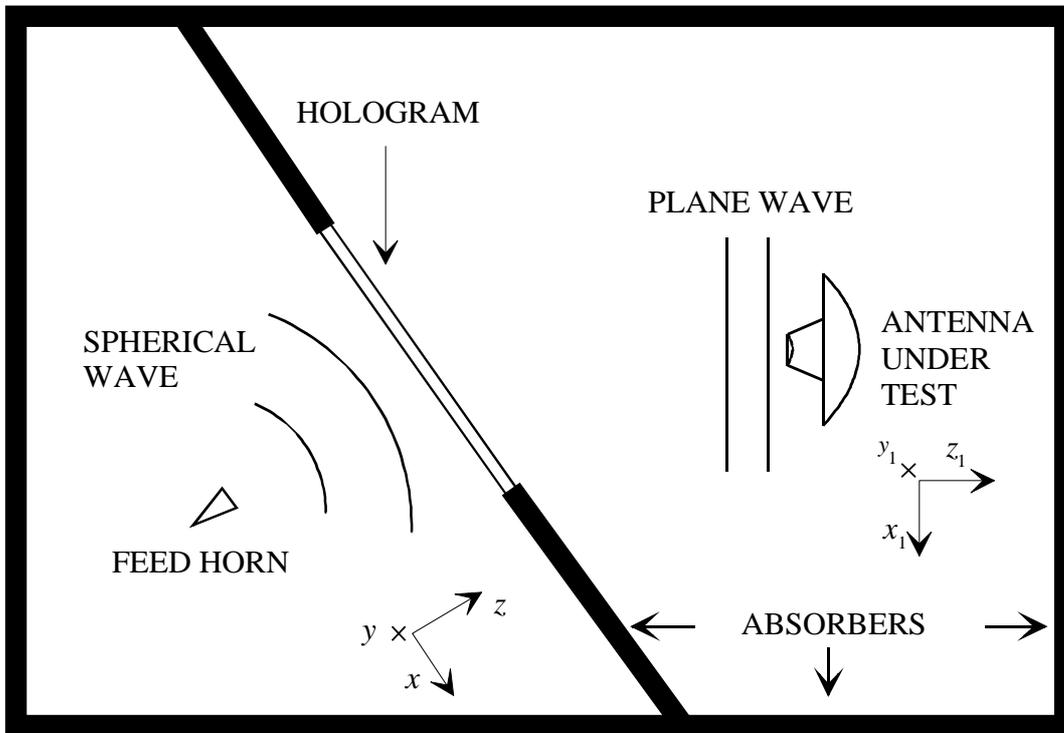
Figure 2.5: Hologram type of a CATR.
