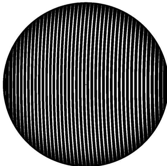
Figure 2.6: Example of a binary amplitude hologram.
