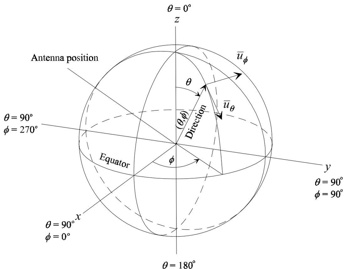
Figure 2.1: Standard spherical coordinate system used in antenna measurements.
