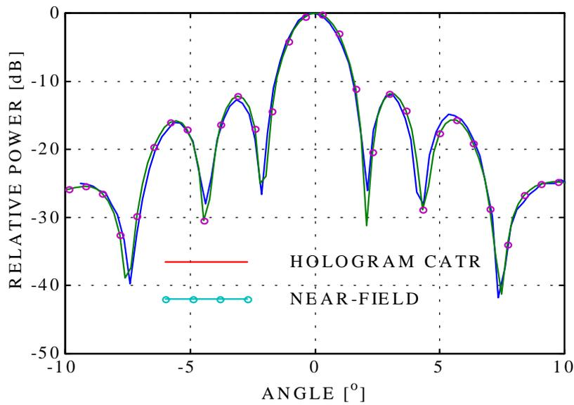
Figure 6. Measured H-plane pattern of a linear array at 40 GHz.
