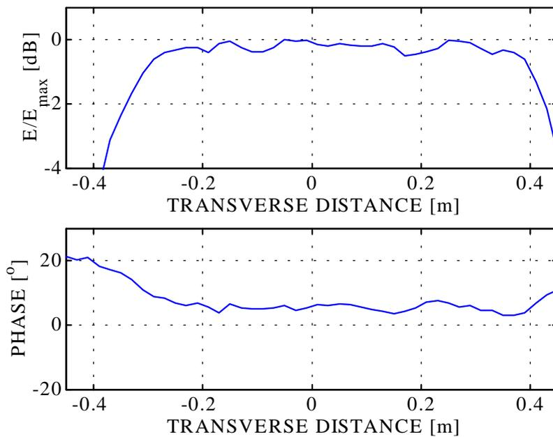
Figure 7. Theoretical transversal quiet-zone field 3.0 m behind the hologram, y-polarization.
