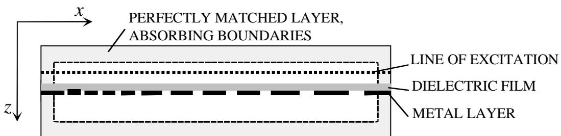
Figure 3. A schematic calculation domain of the FDTD-simulation.
