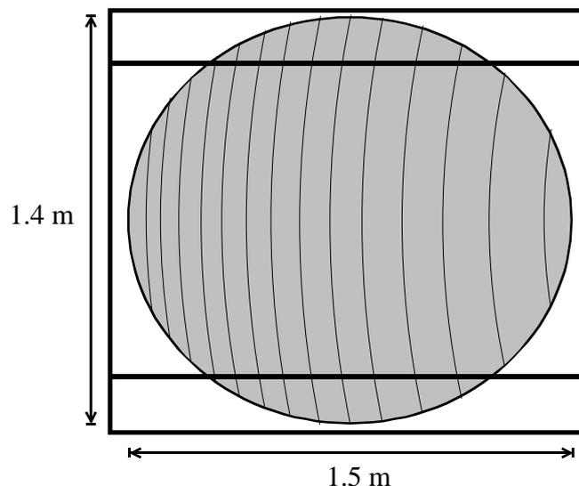
Figure 4. The hologram is joined from three pieces.
