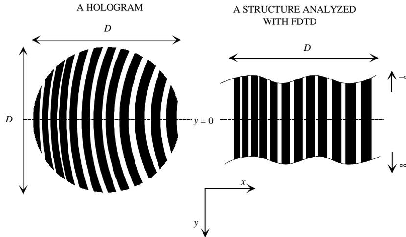
Figure 2. A hologram structure simplification for the simulation.
