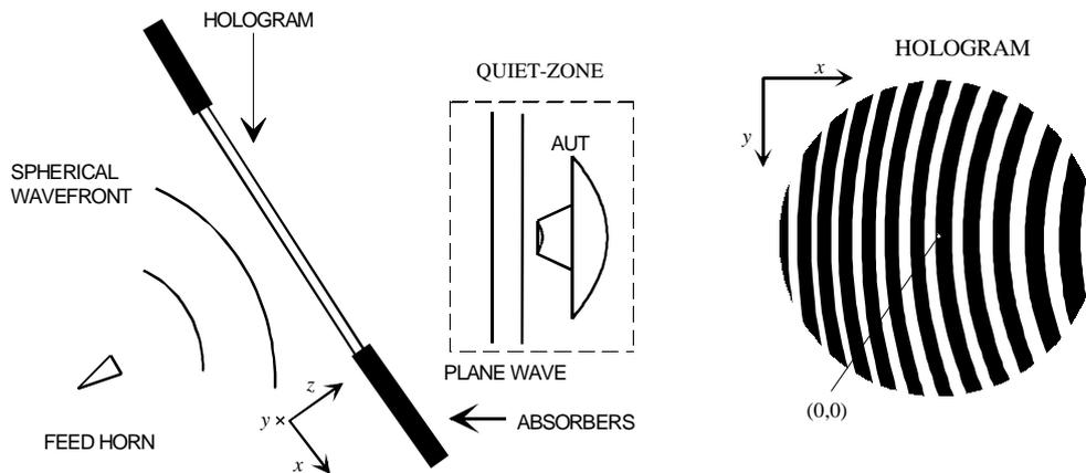
Figure 1. A hologram CATR, and an example of a hologram.
