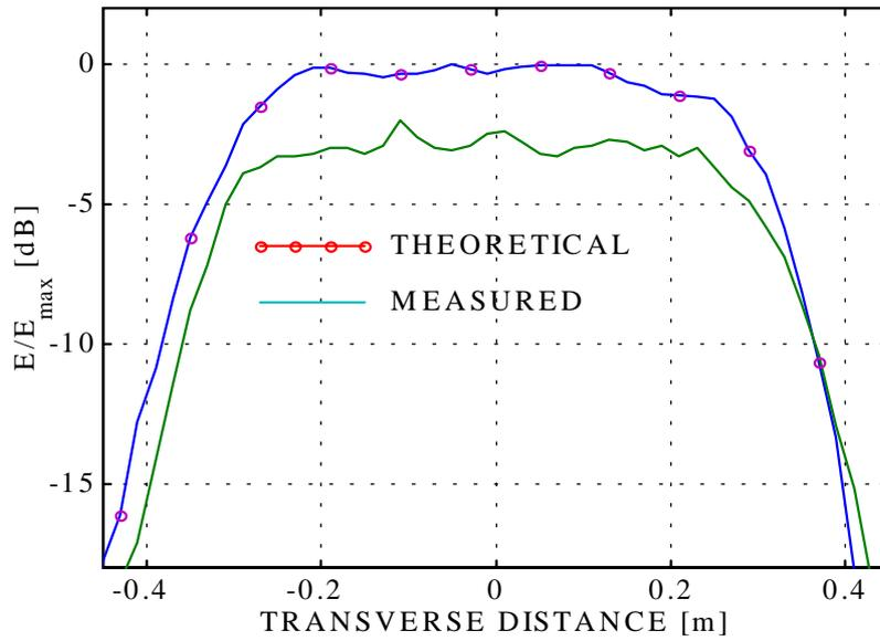
Figure 5. Measured and theoretical transversal quiet-zone fields 3 m behind the hologram, curves are shifted.
