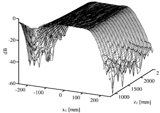
Fig. 9. Theoretical quiet-zone field amplitude in the  $x_1 z_1$  plane ( $y_1 = 0$ ) 0.8–2.5 m behind the hologram.
