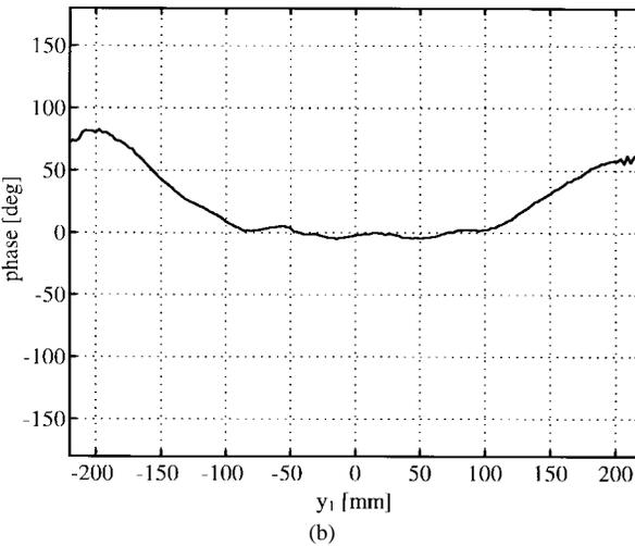
Fig. 7. Measured quiet-zone field in the  $y_1$  direction ( $x_1 = 0$ ) with vertical polarization at 119 GHz.
