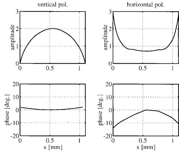
Fig. 4. Aperture electric field in a slot with a vertical and a horizontal polarization.
