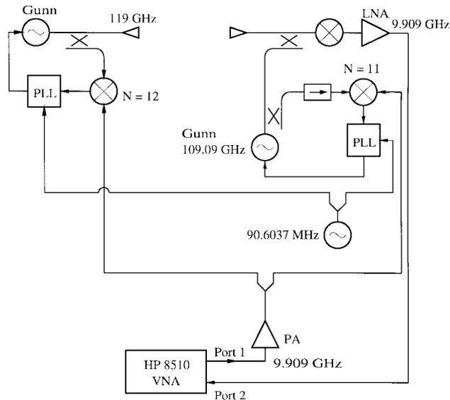
Fig. 5. Measurement setup.
