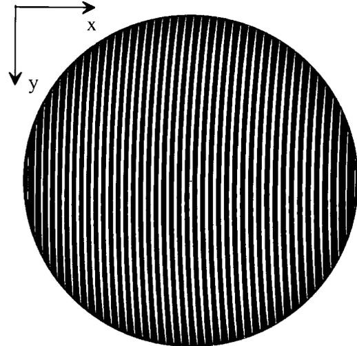
Fig. 2. An example of a binary amplitude hologram pattern. Nontransparent and transparent parts are shown with black and white, respectively.
