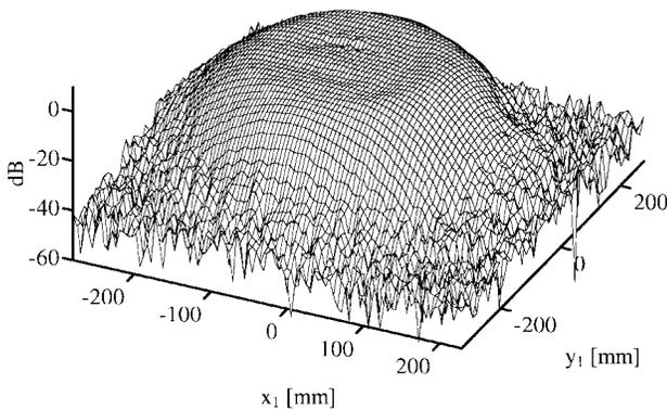
Fig. 8. A three-dimensional (3-D) measurement result of the quiet-zone field amplitude with vertical polarization at 119 GHz.
