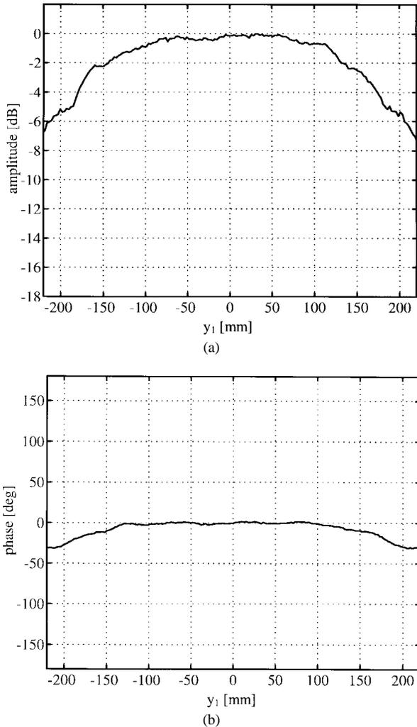
Fig. 11. Measured quiet-zone field in  $y_1$  direction ( $x_1 = 0$ ) with horizontal polarization at 119 GHz.
