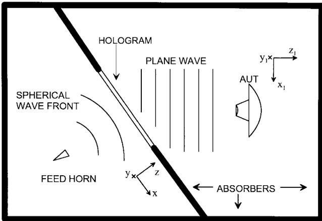
Fig. 1. Measurement arrangement for a hologram CATR.
