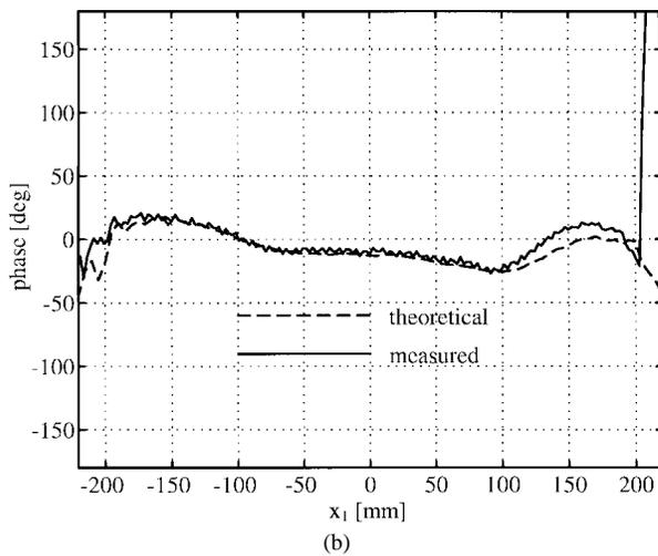
Fig. 6. Theoretical and measured quiet-zone field with a vertical polarization at 119 GHz in the  $x_1$  direction ( $y_1 = 0$ ). The diameter of the hologram is 550 mm.
