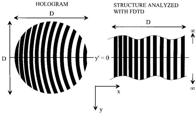
Fig. 3. The structure of the hologram and the structure, which is used in the theoretical analysis.
