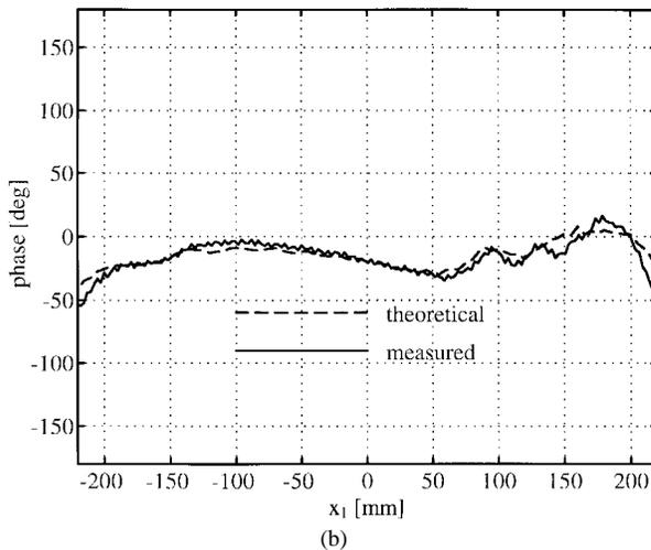
Fig. 10. Theoretical and measured quiet-zone field with horizontal polarization at 119 GHz in the  $x_1$  direction ( $y = 0$ ).
